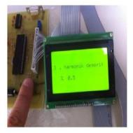
Figure 10 Fundamental component 100% and third harmonic 0.5%
