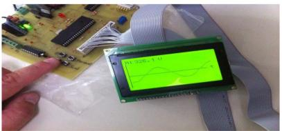
Figure 8. Measurement of city grid voltage harmonics by designed analyzer.
