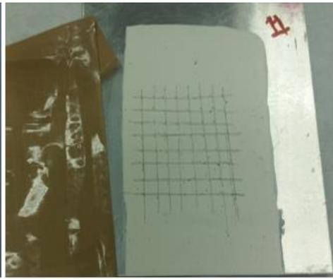
Figure 24. Solvent based paint with aerogel as a paint additive
