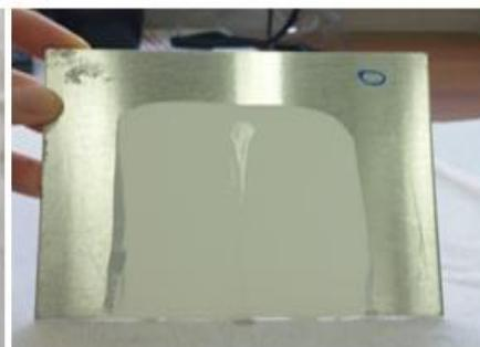
Figure 10. Flow appearance of control sample for water based paint
