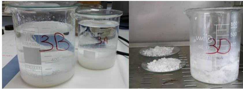
Figure 3. The washing step was done for removing sodium ions.
