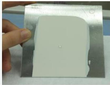
Figure 14. Flow appearance of control sample for solvent based paint
