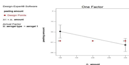
Figure 28. Aerogel amount vs. peeling amount graphic for the solvent based paint
