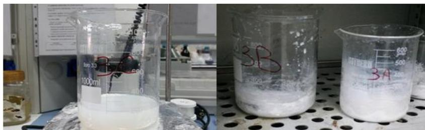
Figure 1. The gelation was occurred after the polymerization step.
