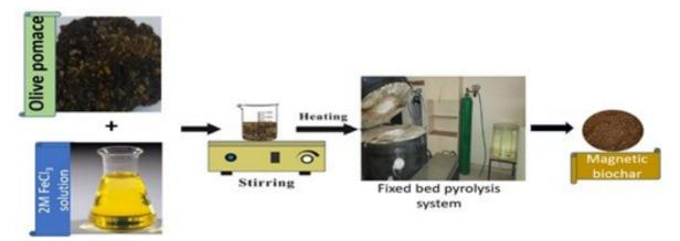
Figure 1. Preparation process of magnetic biochar from OP.
