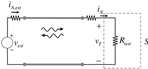
**Figure 8.** Circuit B: a resistor  $R_{test}$  is used to determine  $v_T(t)$  and  $i_N(t)$ , which are to become equivalent sources in an equivalent circuit.
