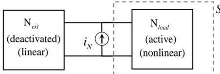
**Figure 3.** The Norton equivalent of the original circuit.
