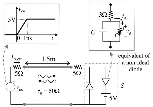
**Figure 7.** Circuit A: a voltage source as shown in the inset is feeding a nonlinear load, which is made up of two diodes and a DC source, via an air filled
