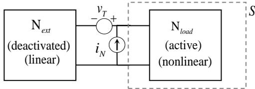
**Figure 6.** Circuit C (a hybrid equivalent circuit). All sources outside  $S$  are switched off, while the Thevenin and Norton sources  $v_T(t)$  and  $i_N(t)$  are placed in the terminals. The time variables are dropped for simplicity.
