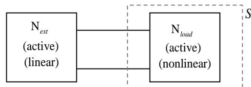
**Figure 4.** Circuit A (the original circuit).  $S$  stands for a closed surface enclosing a network  $N_{load}$ , which may be nonlinear; whereas a network  $N_{ext}$  outside  $S$  is linear.
