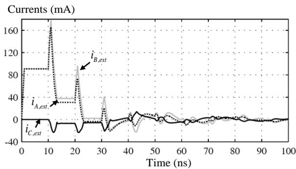
**Figure 12.** The numerical results for the individual currents  $i_{A,ext}(t)$ ,  $i_{B,ext}(t)$ , and  $i_{C,ext}(t)$  in circuits in Figure 7, Figure 10, and Figure 9, respectively. It displays the sum  $i_{B,ext}(t) + i_{C,ext}(t)$  is equal to  $i_{A,ext}(t)$  as claimed by the theorem.
