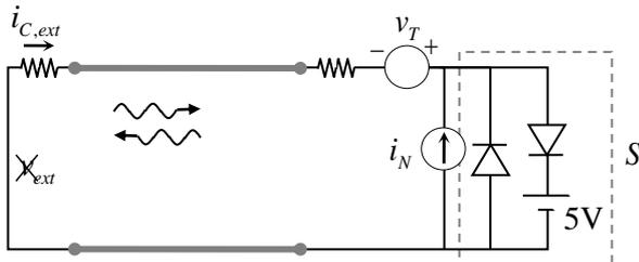
**Figure 9.** Circuit C: the equivalent circuit with the sources  $v_T(t)$  and  $i_N(t)$  at the interface.
