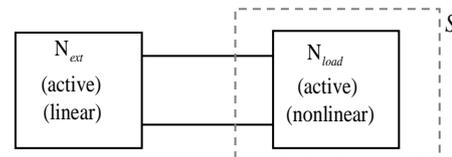
**Figure 1.** The original circuit. It is made up of linear components except some components inside  $S$ , which may be nonlinear.
