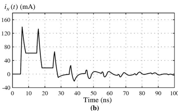
**Figure 11.** (a) The Thevenin voltage  $v_T(t)$  versus  $t$  according to the case inside  $S$  in Figure 10. (b) The Norton current  $i_N(t)$  versus  $t$  according to the case inside  $S$  in Figure 10.
