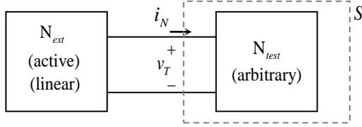
**Figure 5.** Circuit B (a test setup). It is for determining the sources  $v_T(t)$  and  $i_N(t)$ . The network  $N_{load}$  has been replaced by an arbitrarily chosen  $N_{test}$ .
