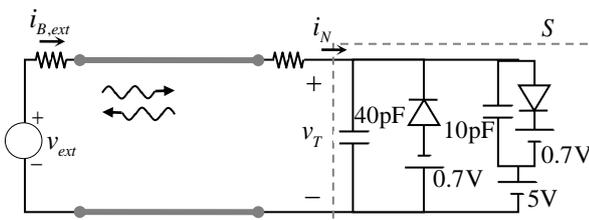
**Figure 10.** Circuit B: some arbitrarily chosen capacitors, sources, and diodes are placed inside  $S$ .
