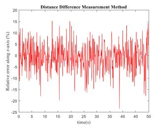
**Fig. 10**. Relative error along the z-axis when using the distance difference measurement method.
