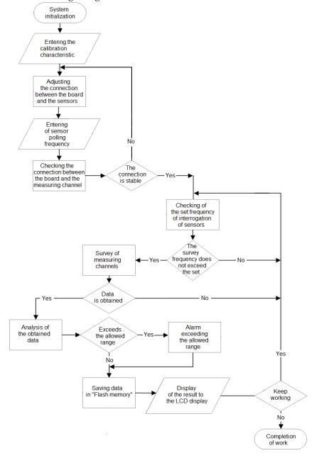
Fig. 4. Algorithm of measurement system operation
