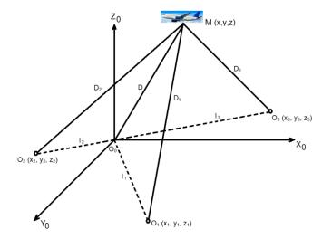
Fig. 2. Distance measurement method's scheme in determining the position of the aircraft
