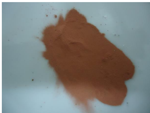
Fig 2. Metallic copper powder obtained after copper ions reduction
