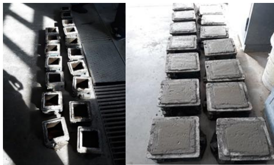
Picture 1. Molds where samples are poured and their appearance after pouring
