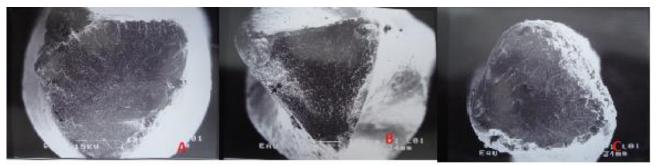
Figure 3. Image of covered instruments after test procedures A: HeroShaper, B: Race, and C: TF
