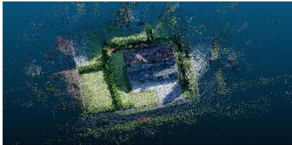
FIGURE 12. Concatenated point cloud using ICP algorithm.
