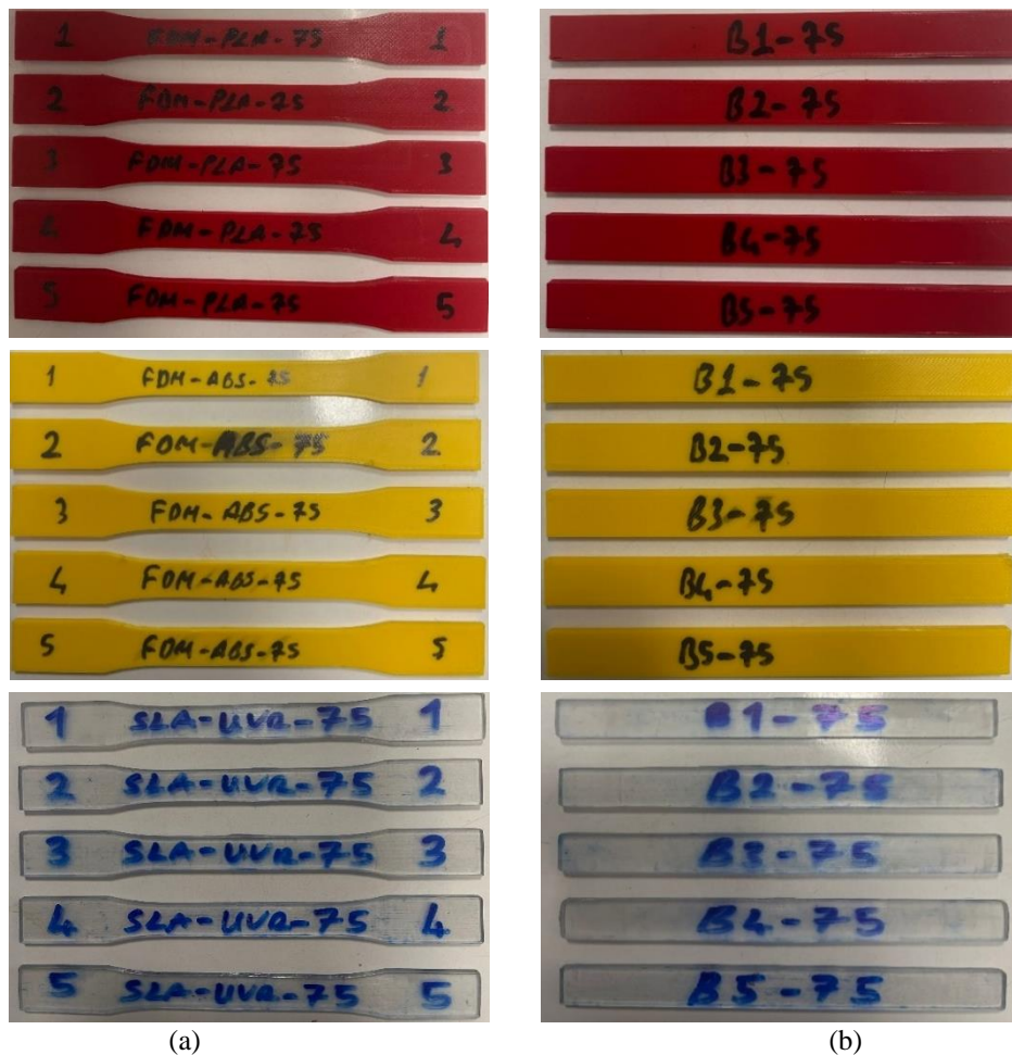
Figure 3. Tensile and 3-point bending test specimens fabricated on a 3D printer using PLA, ABS and UVR materials: (a) Tensile test specimens (b) 3-point bending test specimens
