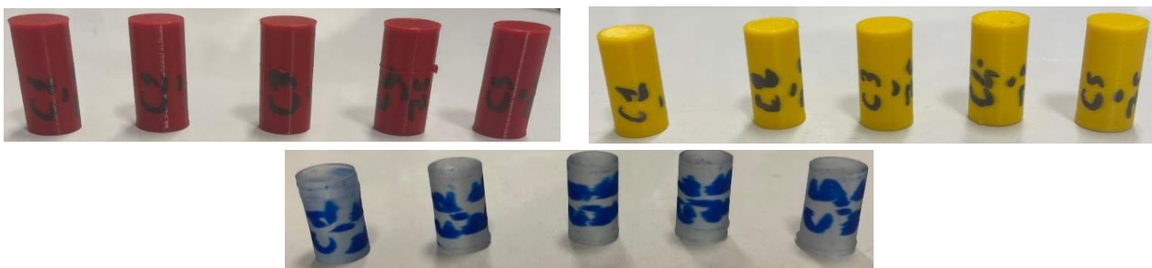
Figure 4. Compression test samples fabricated on a 3D printer using PLA, ABS and UVR materials
