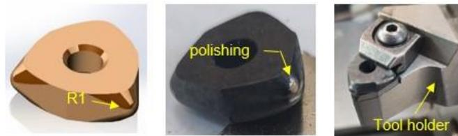
**Figure 2.** Designed insert, its manufacturing and assembling on the tool holder
