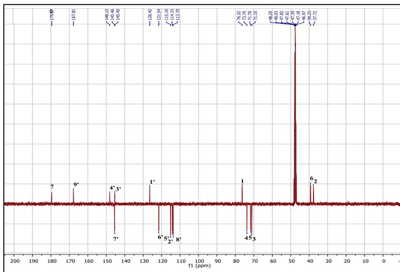
**Figure 3.**  $^{13}\text{C-APT}$  NMR Spectrum of chlorogenic acid ( $\text{CD}_3\text{OD}$ , 100 MHz).
