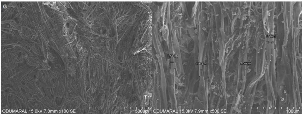
**Figure 1G.** The outer surface of the section and thickness of the fibers the nestwall of *V. crabro*.
