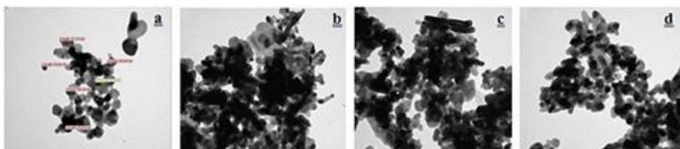
**Figure 1.** TEM micrograph of dispersion and dispersion of ZnO suspension at four different concentrations (250, 500, 1000, 2000 mgL<sup>-1</sup>). (x 300000) (a) 250 mgL<sup>-1</sup>, (b) 500 mgL<sup>-1</sup> particle aggregation, (c) 1000 mgL<sup>-1</sup> particle aggregation, (d) 2000 mgL<sup>-1</sup> particle aggregation.
