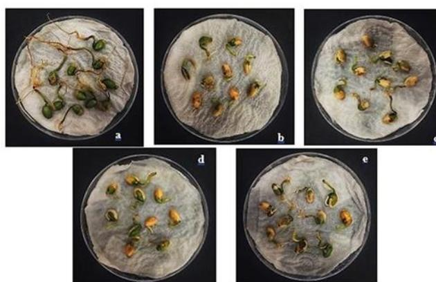
**Figure 4.** Effect of ZnO nanoparticle on germination percentage of soya bean seeds at the end of 96th hour **a:** control, **b:** 250 mgL<sup>-1</sup>, **c:** 500 mgL<sup>-1</sup>, **d:** 1000 mgL<sup>-1</sup>, **e:** 2000 mgL<sup>-1</sup>.
