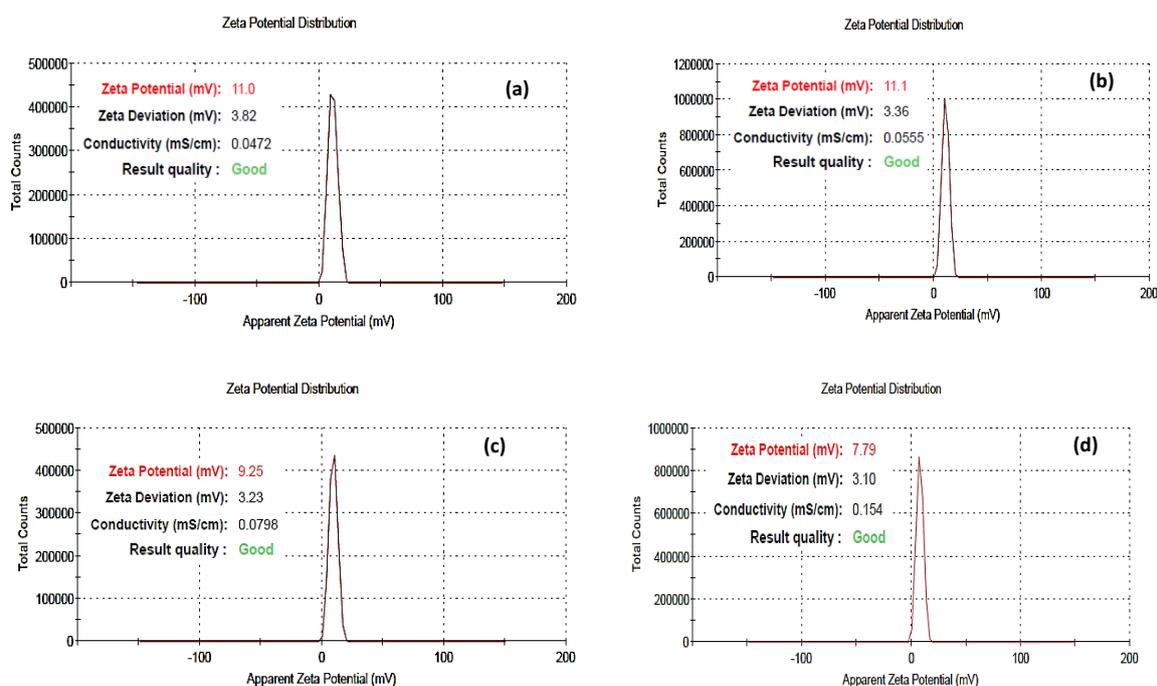
**Figure 2.** Zeta potential values of ZnO suspension at four different concentrations (250, 500, 1000, 2000 mgL<sup>-1</sup>). (a) 250 mgL<sup>-1</sup>, (b) 500 mgL<sup>-1</sup>, (c) 1000 mgL<sup>-1</sup>, (d) 2000 mgL<sup>-1</sup>.
