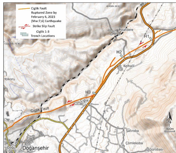
Figure Surface fault-rupture of the February 6, 2023 ( M_w : 7.6) earthquake mapped between Dogansehir and Eskikoy on the topographic map
