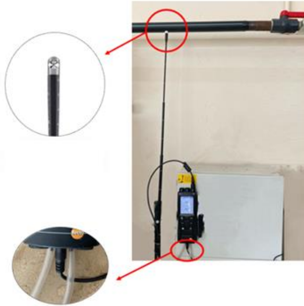
Figure 2. Digital air velocity and differential pressure meter.
