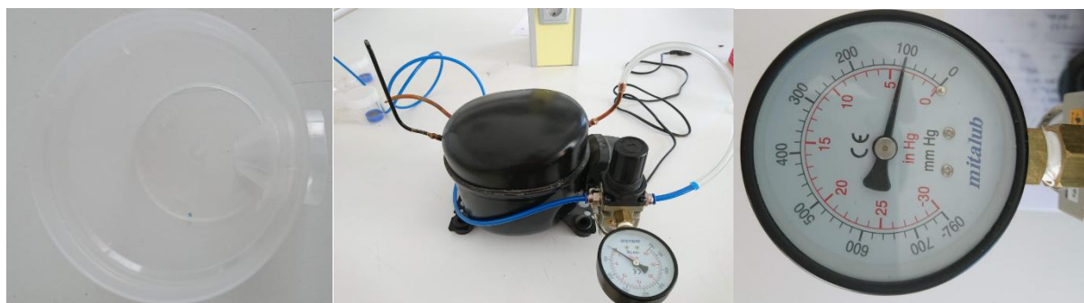
Fig 2 Lidded plastic container designed to be funnel-shaped for storing manures (left), the vacuum pump (middle), and vacuum pump's suction pressure (right)
