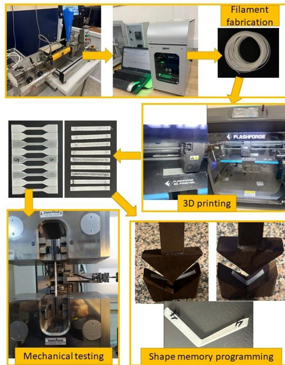
Figure 4. Experimental setup and workflow of the study
