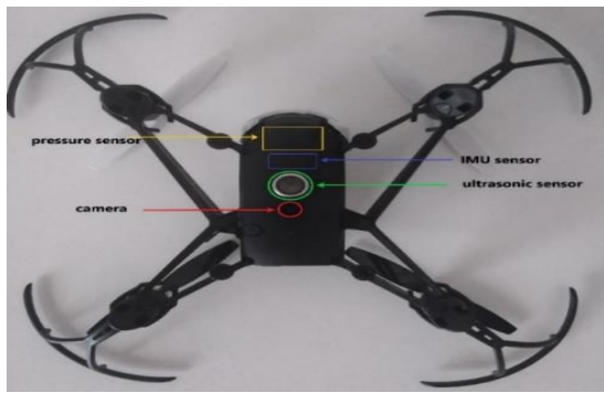
Figure 5. Illustration of sensors on the quadrotor [18].
