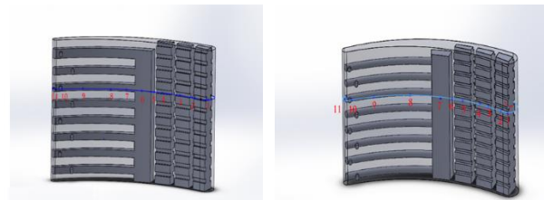
Figure 6. The design of internal cooling channels for first and enhanced design.
