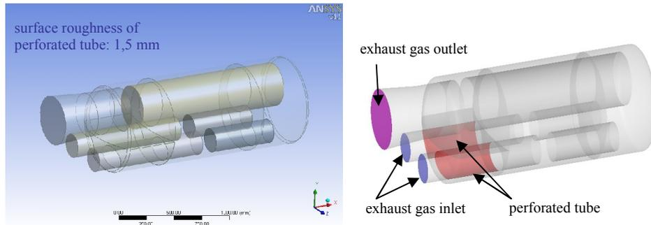
Figure-1: First Dry-Type Silencer Model
