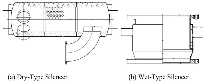
Figure-15: Technical Drawings Belonging to Dry and Wet-Type Silencers [6]
