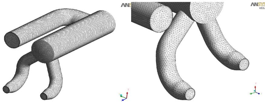
Figure-4: Modified Dry-Type Silencer Model Mesh (Geometry-2)
