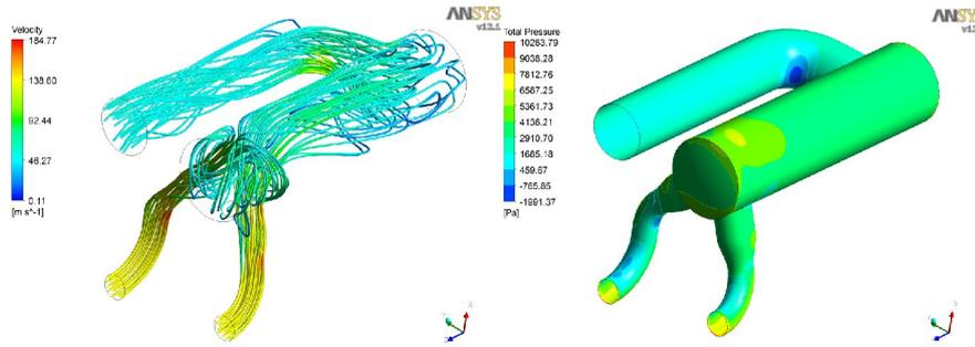
Figure-5: Stream Lines and Pressure Loss (Geometry-1)
