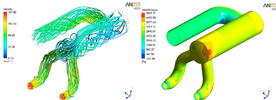
Figure-6: Stream Lines and Pressure Loss (Geometry-2)
