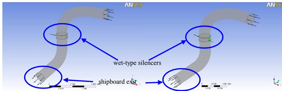
(a) Single Inlet (perp. and 45° inclined ) (b) Double Inlet (perp. and 45° inclined )
