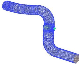
Figure-10: Wet-Type Silencer Model Mesh
