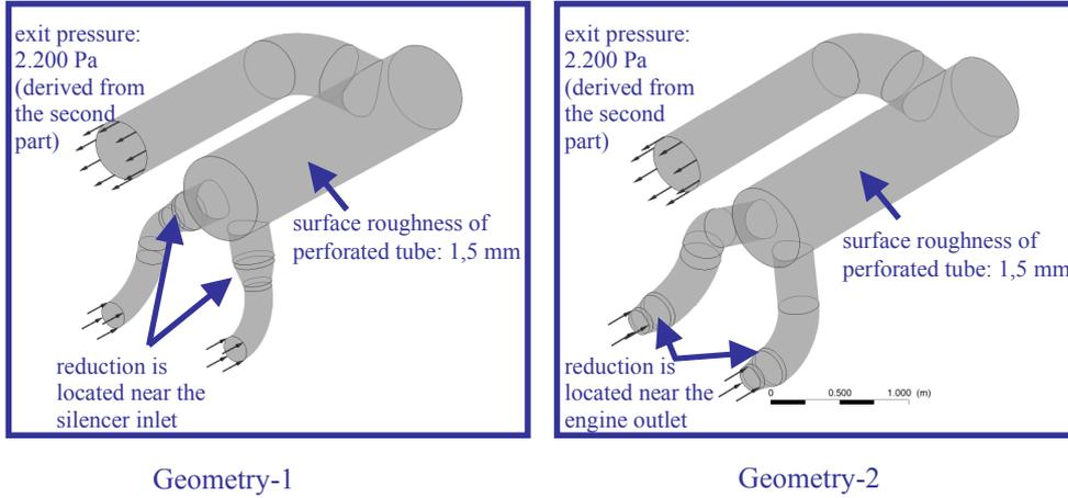
Figure-3: Modified Dry-Type Silencer Models
