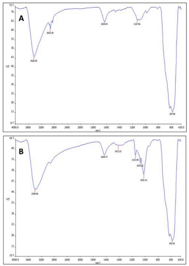
Figure 1. FTIR spectra of A) pure magnetite and B) starch coated magnetic nanoparticles.
