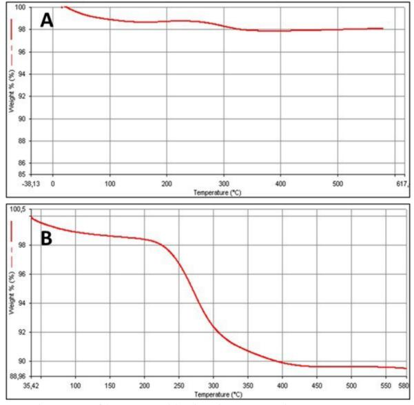
Figure 2. Themogram curves of A) pure magnetite and B) starch coated magnetic nanoparticles.
