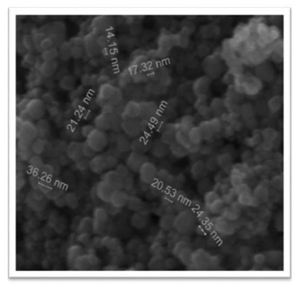
Figure 3. SEM images of starch coated magnetic nanoparticles.
