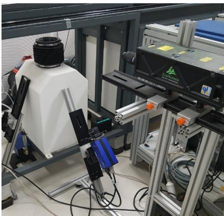
**Figure 7.** 2D PIV test setup PIV
