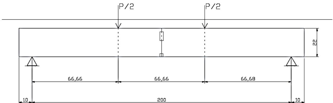
**Figure 1.** Loading scheme of the beams
