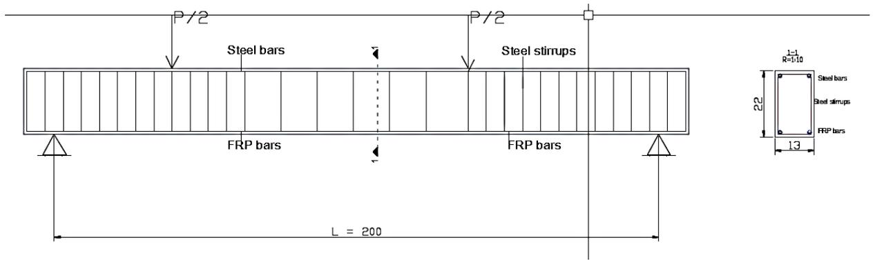
**Figure 2.** Type of reinforcement used for beams
