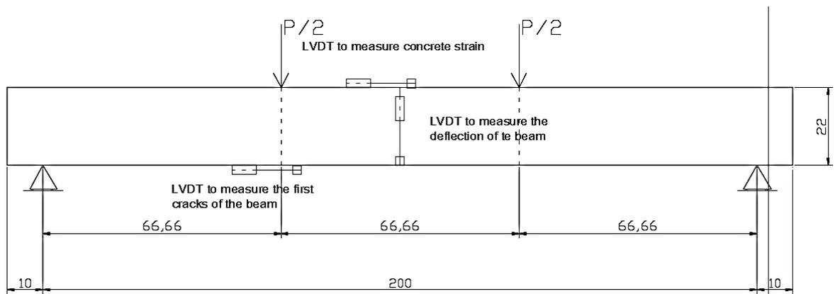
**Figure 3.** The way of installing the instrumentation LVDT
