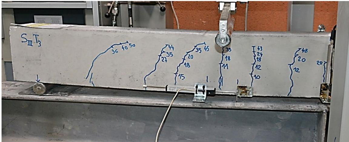
**Figure 4.** Cracks in the surface of the beam
