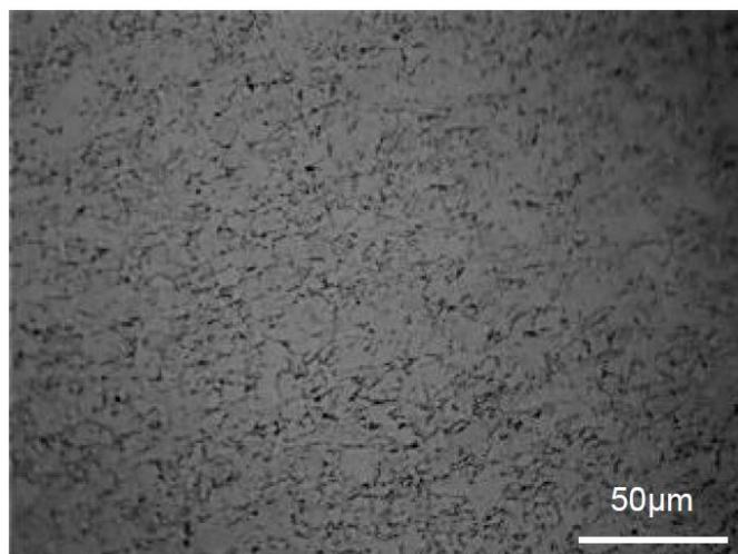
**Figure 4.** Microstructure of the base metal (X70 steel)
