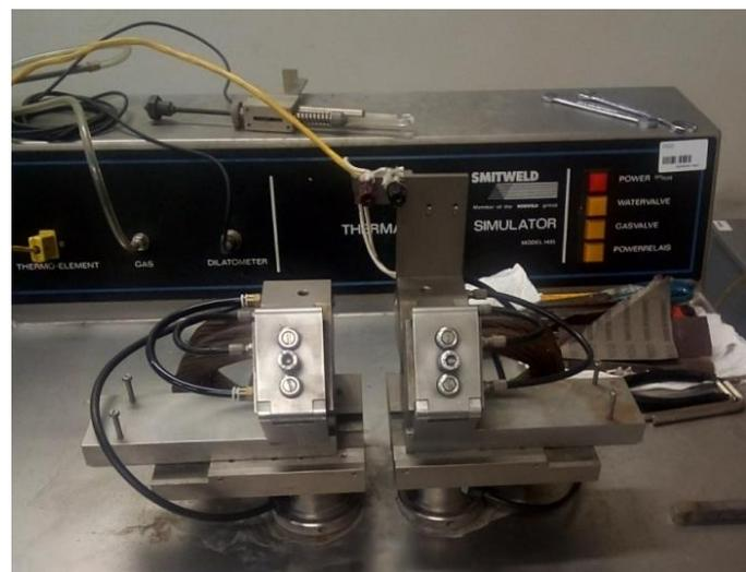
**Figure 1.** Smitweld thermal cycle simulator
