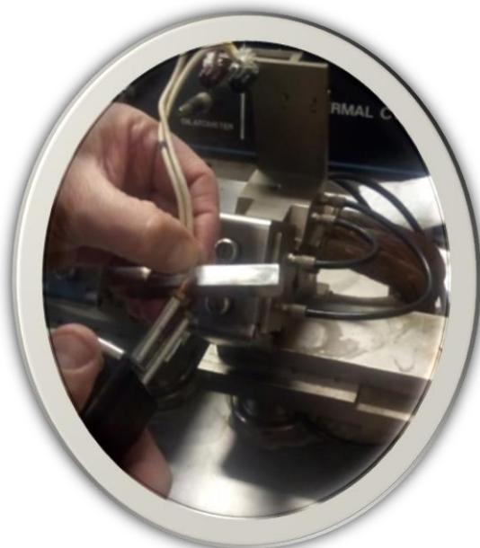
**Figure 3.** Fixing of the thermocouple on the standardized test specimen
