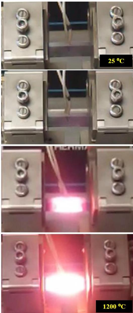
**Figure 5.** Effect of heat treatment on specimen of X70 steel during heating from 25 °C to 1200 °C
