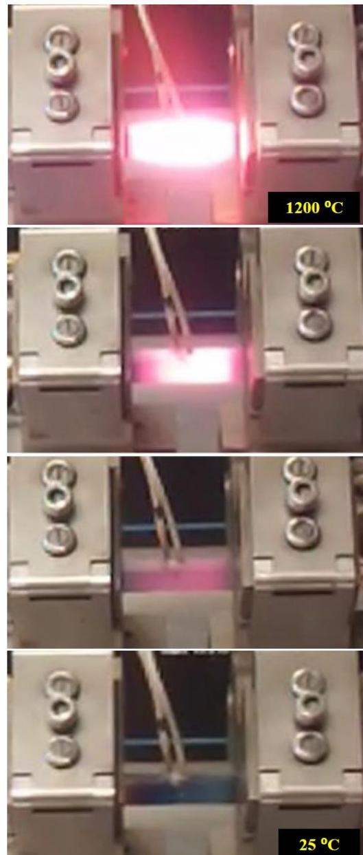
**Figure 6.** Thermal behavior of X70 steel during cooling process from 1200 to 25 °C
