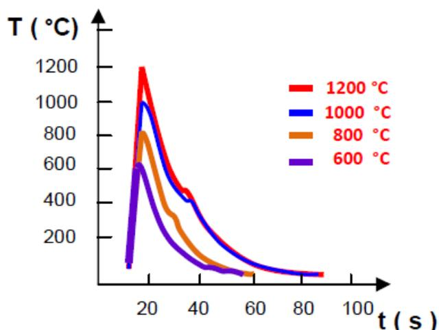
**Figure 2.** Thermal cycles applied to the specimen.
