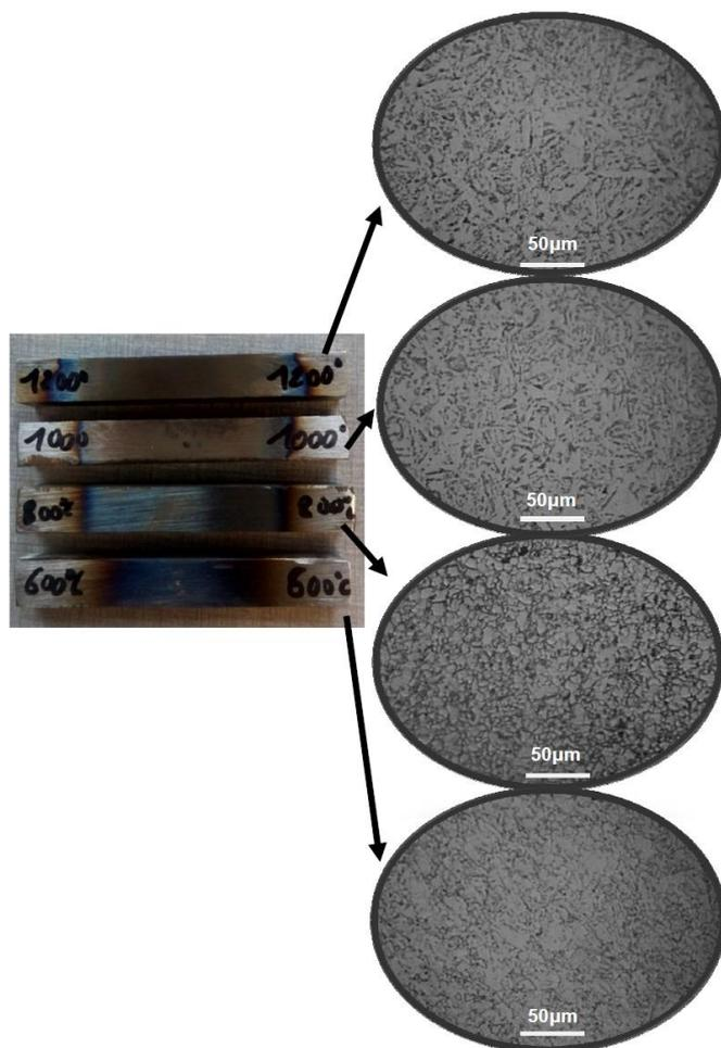
**Figure 7.** View of X70 steel specimens after different thermal cycles (600, 800, 1000 and 1200°C) with their microstructures
