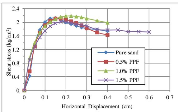
Figure 8. Shear box test results for sand and PPF-reinforced sand at normal stress of 1.667 kg/cm<sup>2</sup>.
