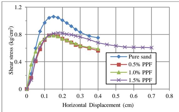
Figure 6. Shear box test results for sand and PPF-reinforced sand at a normal stress of 0.556 kg/cm<sup>2</sup>.
