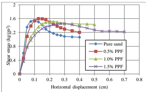
Figure 7. Shear box test results for sand and PPF-reinforced sand at normal stress of 1.111 kg/cm<sup>2</sup>.
