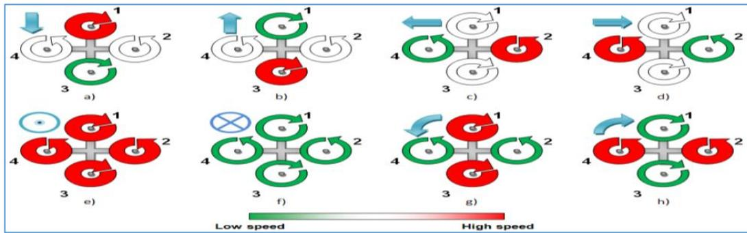
Figure 3. Various directions of movement of the quadcopter [9]
