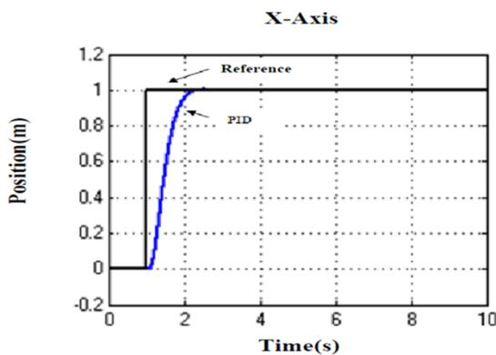
Figure 5: PID simulation model and simulation result for x-axis ( $m=0.964$  kg,  $I_{xx} = 8.5532 \times 10^{-3}$  kgm<sup>2</sup>,  $x_{ref} = 1$  m)
