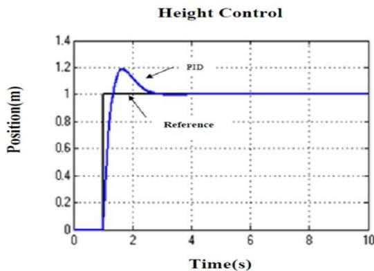
Figure 4: PID simulation model and simulation result for height ( $m=0.964$  kg,  $g=9.8$  m/s<sup>2</sup>)
