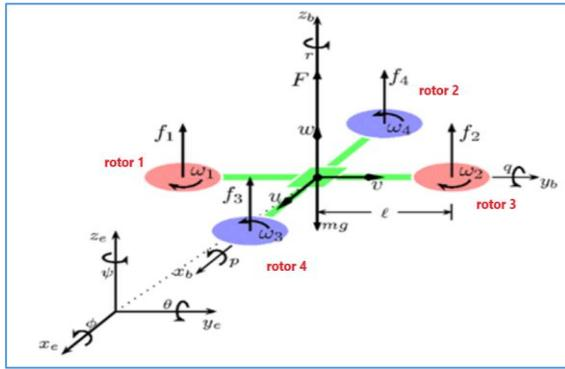
Figure 2: Rotation directions of quadcopter rotors
