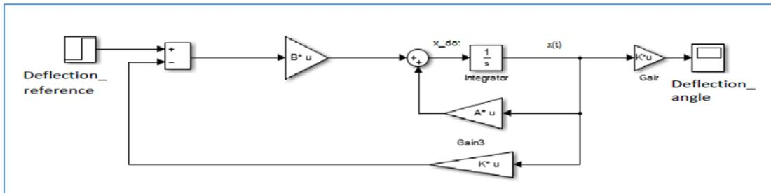
Figure 9: LQR simulation model for deflection angle.
