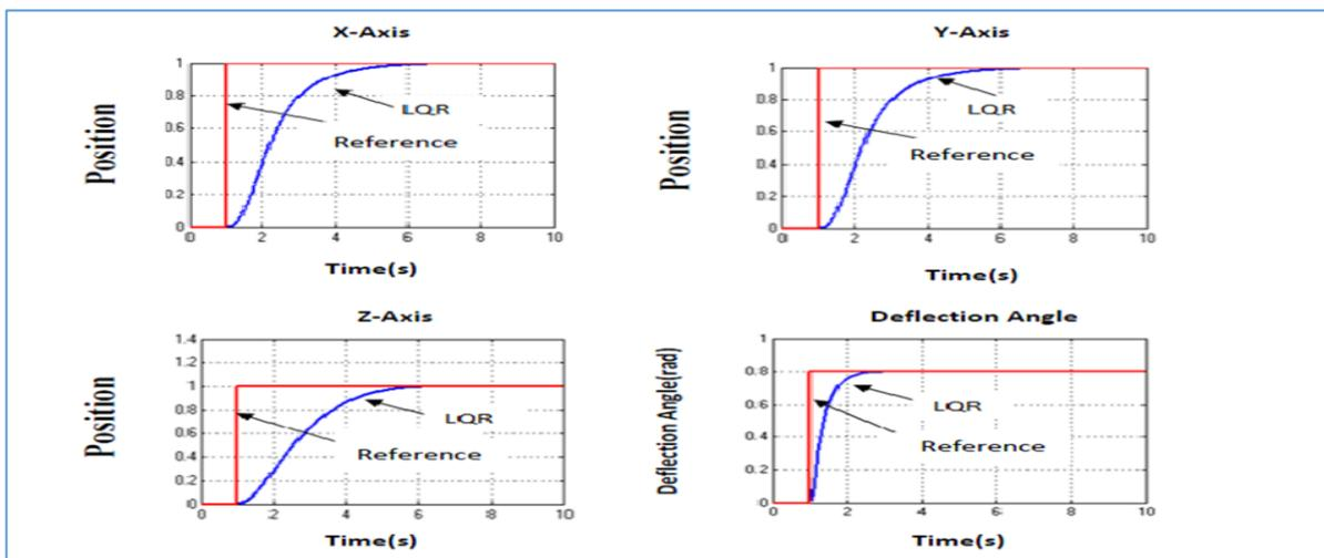
Figure 10: LQR Control simulation results
