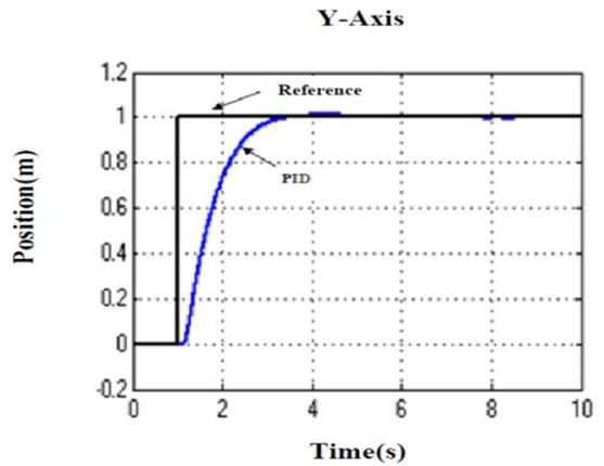
Figure 6: PID simulation model and simulation result for y-axis ( $m=0.964$  kg,  $I_{yy} = 8.5532 \times 10^{-3}$  kgm<sup>2</sup>,  $y_{ref} = 1$  m)
