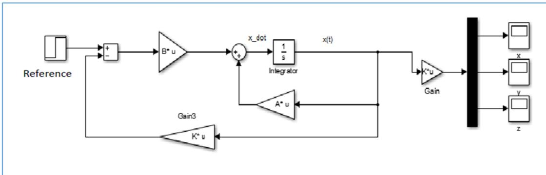
Figure 8: LQR simulation model for x, y, z axes
