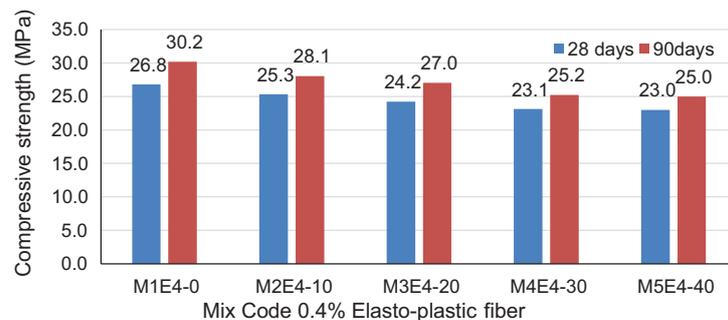
**Figure 1.** Compressive strength results.
