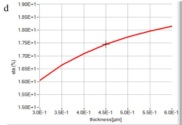
Figure 3 Variation of (a) open-circuit voltage (b) short-circuit current (c) fill-factor (d) power conversion efficiency (eta) by the increment of absorber thickness
