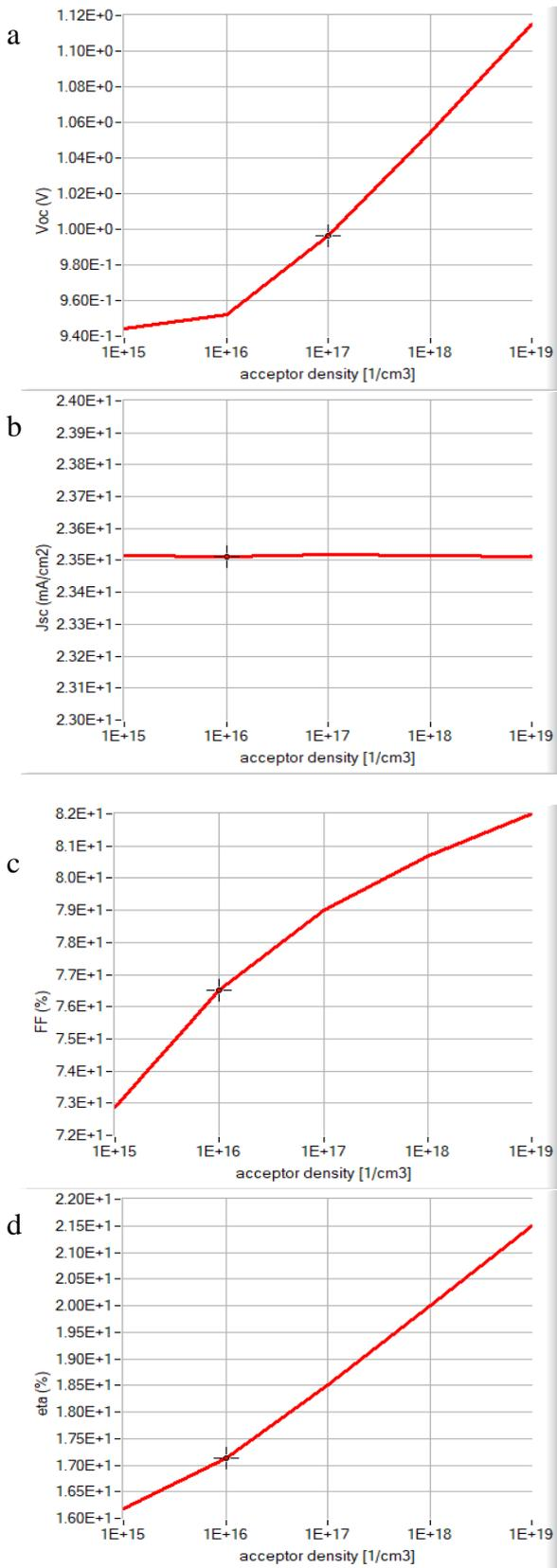
Figure 6 Variation of (a) open-circuit voltage (b) short-circuit current (c) fill-factor (d) power
