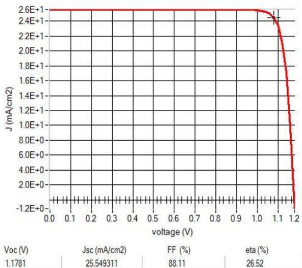
Figure 10 The final current-voltage curve of the modified cell by the optimized parameters
