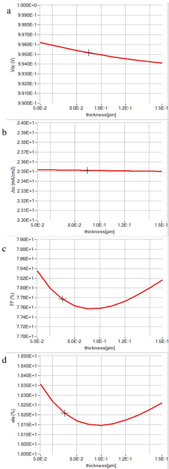
Figure 4 Variation of (a) open-circuit voltage (b) short-circuit current (c) fill-factor (d) power conversion efficiency by the increment of ETM thickness
