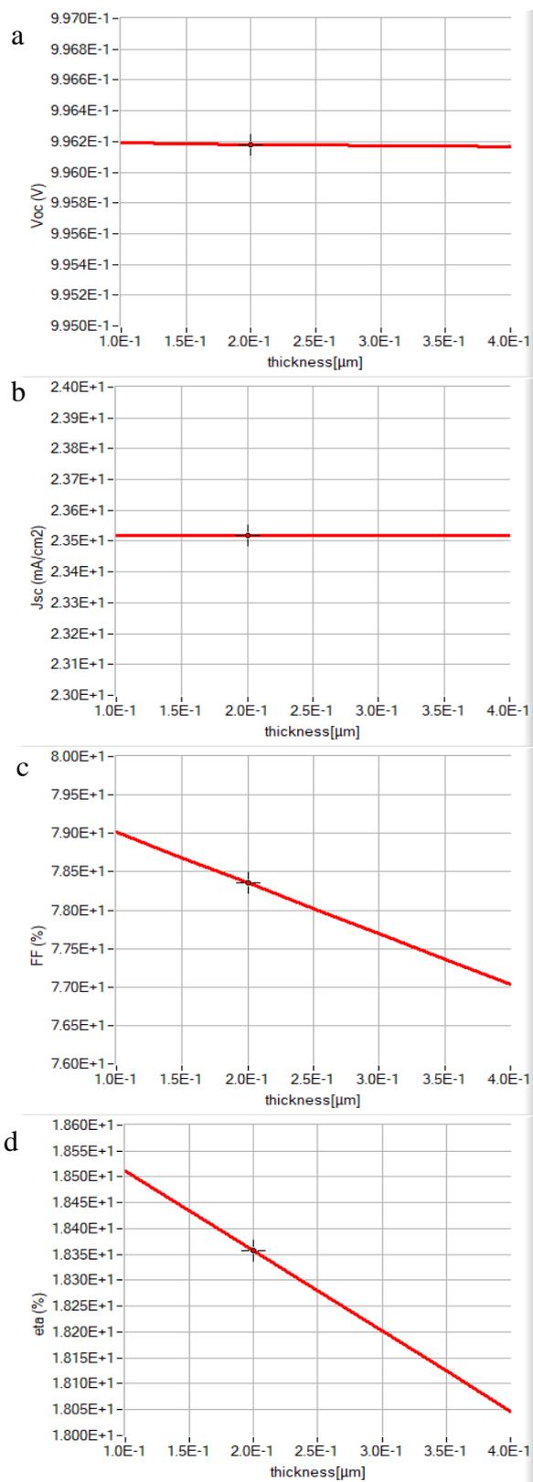
Figure 5 Variation of (a) open-circuit voltage (b) short-circuit current (c) fill-factor (d) power conversion efficiency (eta) by the increment of HTM thickness
