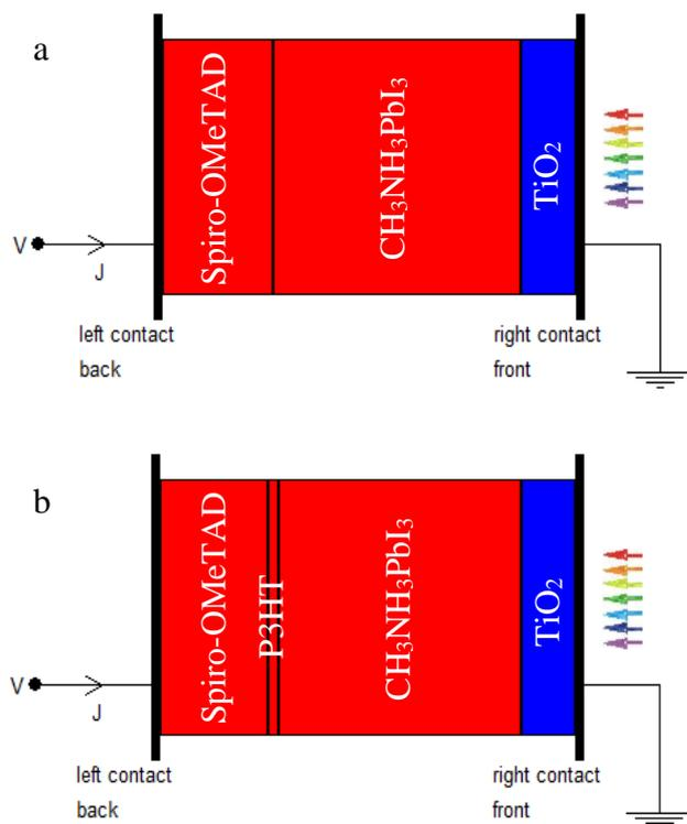
Figure 2 Perovskite solar cell (a) simple (b) modified structure used in this work
