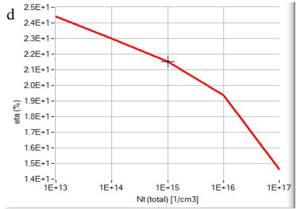
Figure 9 Variation of (a) open-circuit voltage (b) short-circuit current (c) fill-factor (d) power conversion efficiency by the increment of defect density of the absorber
