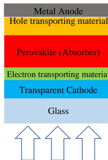
Figure 1 Perovskite solar cell's general structure [1]
