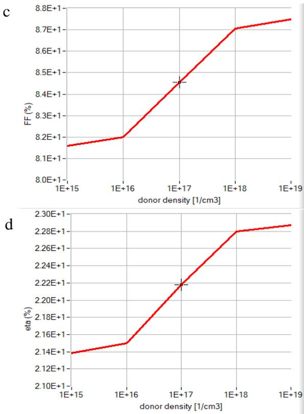
Figure 7 Variation of (a) open-circuit voltage (b) short-circuit current (c) fill-factor (d) power conversion efficiency (eta) by the increment of dopant concentrations of ETM
