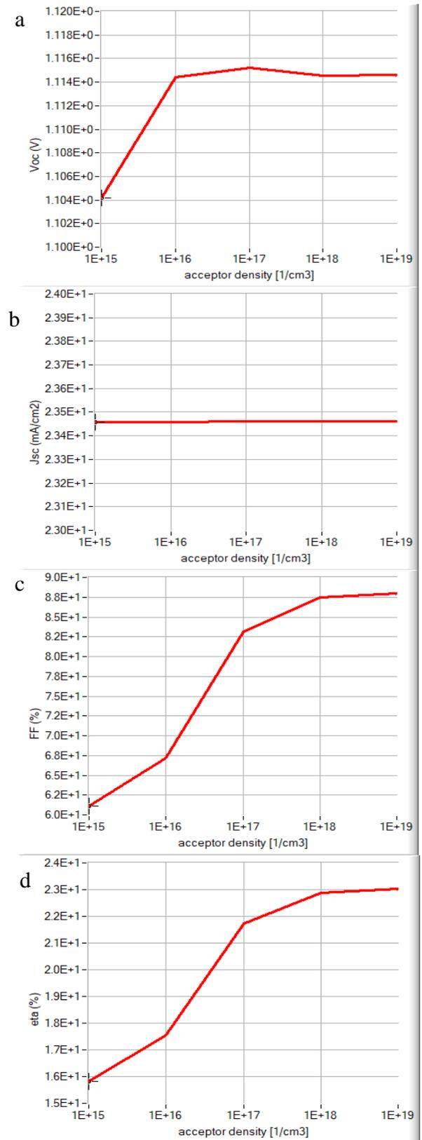
Figure 8 Variation of (a) open-circuit voltage (b) short-circuit current (c) fill-factor (d) power conversion efficiency (eta) by the increment of dopant concentrations of HTM
