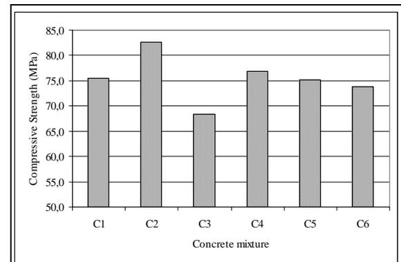
Figure 1. 28 day compressive strength test results.
