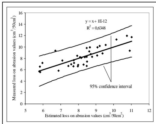
Figure 4. Comparison of experimental and calculated loss on abrasion values
