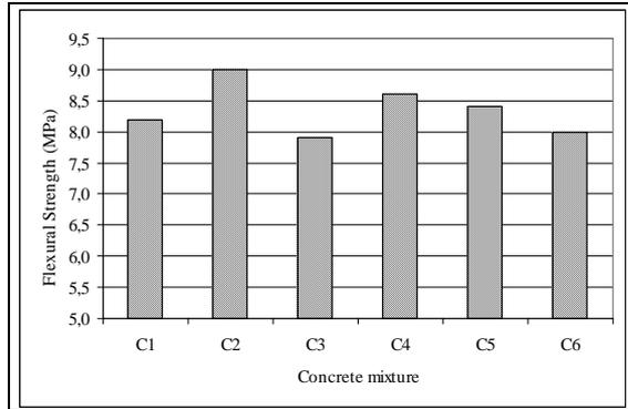
Figure 2. 28 day flexural strength test results
