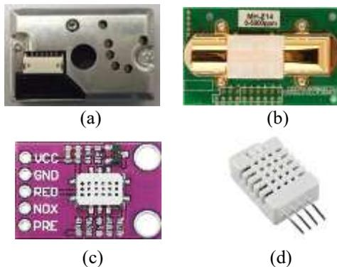
**Fig. 2.** The sensor array used in the proposed e-nose system; a) GP2Y1010AU, b) MH-Z14, c) MICS-4514, d) DHT22.
