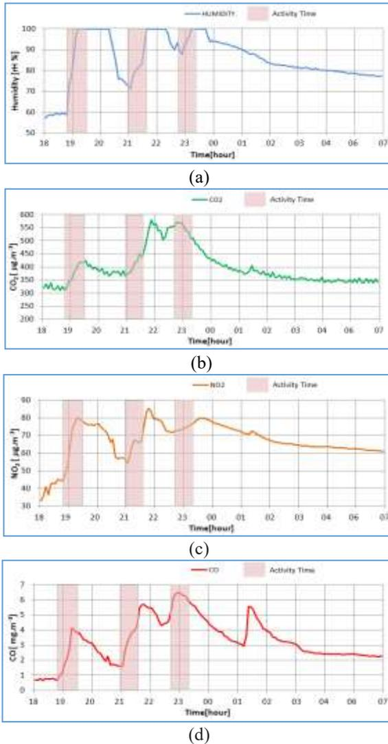
**Fig.5.** Air Quality Data of Shower Activity a) Humidity, b) CO<sub>2</sub>, c) NO<sub>2</sub>, d) CO
