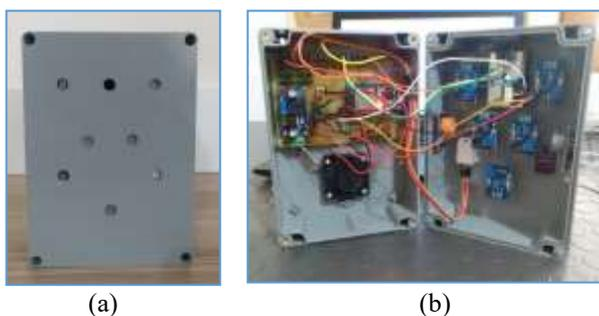
**Fig. 3.** IoT based e-nose measurement system a) Outer view, b) Interior view.
