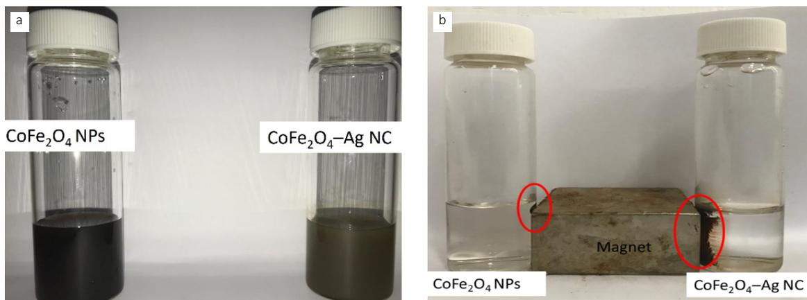
**Figure 3.** a) Color differences between  $\text{CoFe}_2\text{O}_4$  NPs and  $\text{CoFe}_2\text{O}_4$ -Ag NCs. (5<sup>th</sup> sample) b) Behaviors of  $\text{CoFe}_2\text{O}_4$  NPs and  $\text{CoFe}_2\text{O}_4$ -Ag NCs. (5<sup>th</sup> sample) under the magnetic field after 10 minutes later.
