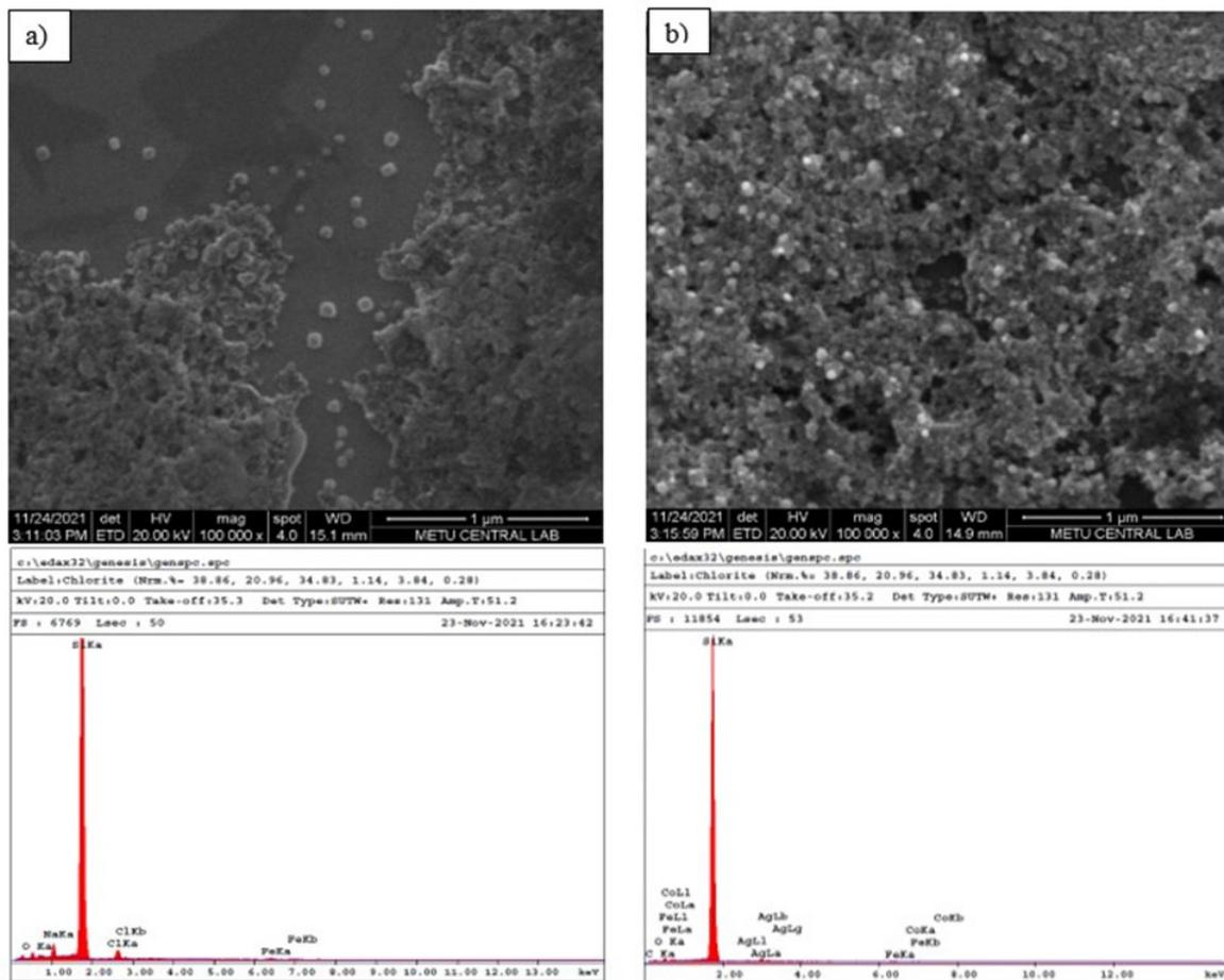
Figure 5. a) SEM images and EDX pattern of CoFe<sub>2</sub>O<sub>4</sub> NPs b) SEM images and EDX pattern of CoFe<sub>2</sub>O<sub>4</sub>-Ag NCs.
