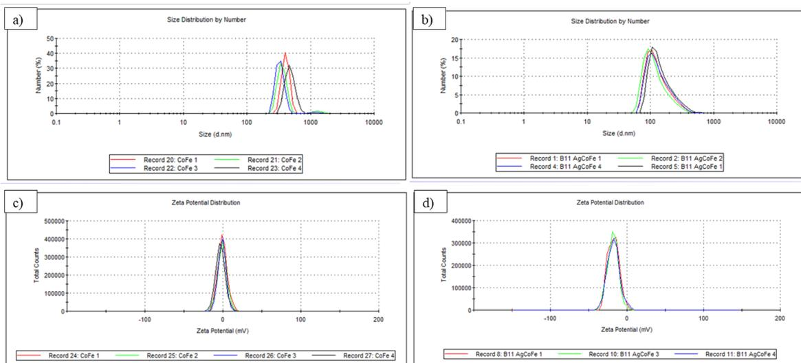
Figure 6. DLS measurement of the number average size of a) CoFe<sub>2</sub>O<sub>4</sub> NPs and b) CoFe<sub>2</sub>O<sub>4</sub>-Ag NCs. Zeta measurements of c) CoFe<sub>2</sub>O<sub>4</sub> NPs and d) CoFe<sub>2</sub>O<sub>4</sub>-Ag NCs.
