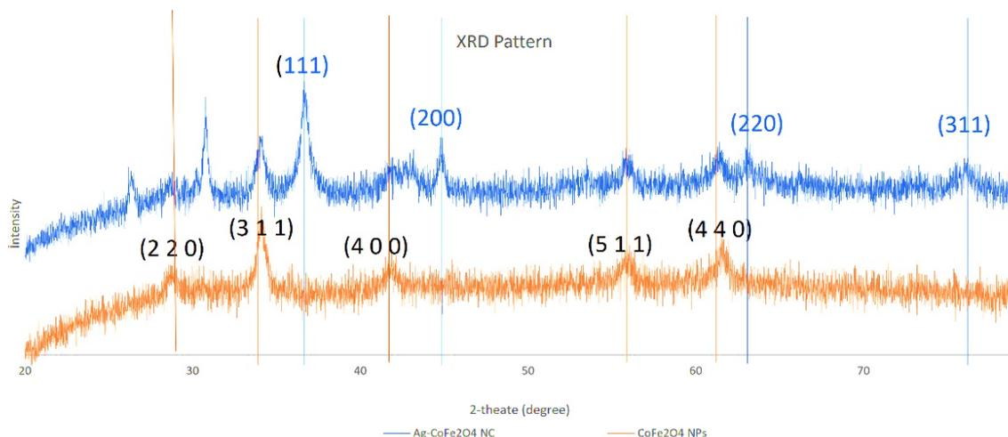
**Figure 4.** The XRD pattern  $\text{CoFe}_2\text{O}_4$ -Ag NC (blue line) and  $\text{CoFe}_2\text{O}_4$  NPs (orange line).
