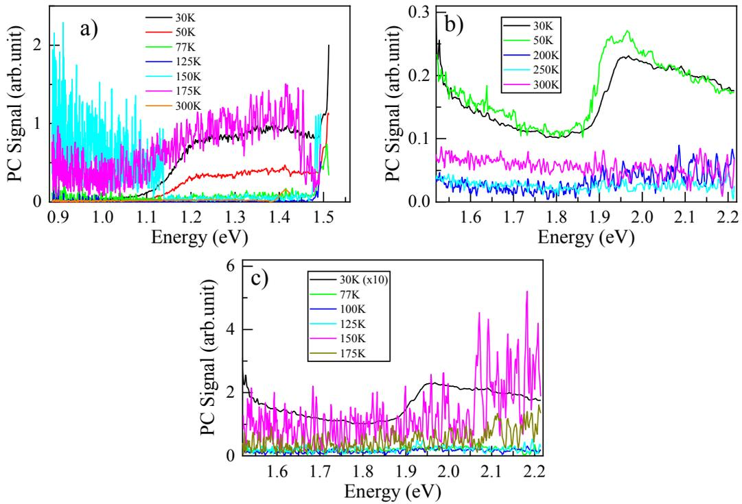
**Figure 3.** Temperature dependent normalized PC spectra of the sample. a) low energy region spectra taken with low pass bandedge filter (cut-on 715 nm). b) high energy region spectra taken with high pass bandedge filter (cut-on 560 nm). c) high energy region spectra taken with high pass bandedge filter (cut-on 560 nm). For comparison, 30 K result in Figure c) is multiplied by 10.
