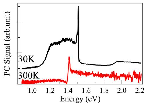
**Figure 2.** Normalized PC spectra of the sample at 30 and 300 K. Black and red colours depict the results for 30 and 300 K, respectively.
