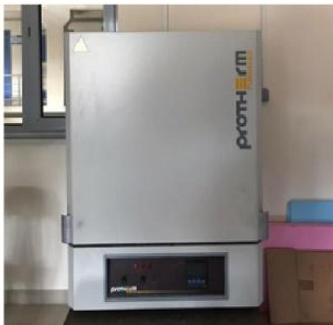
**Figure 3.** Protherm metal furnace.
