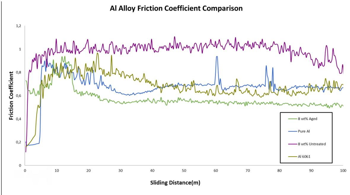
**Figure 5.** Friction coefficients change with sliding distance.
