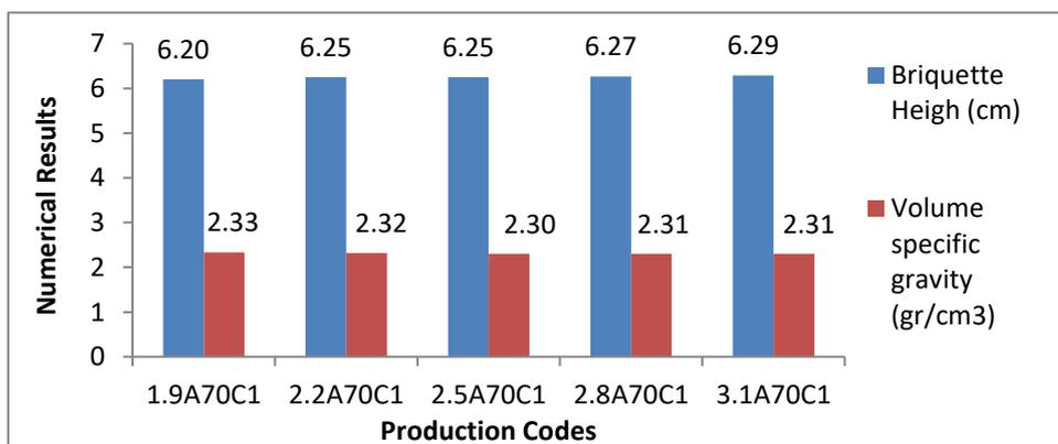
Figure 6. Comparison of briquette height and volume specific gravity values for different bitumen percentages
