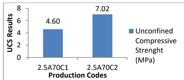
Figure 13. Comparison of unconfined compressive strength values for different cement percentages
