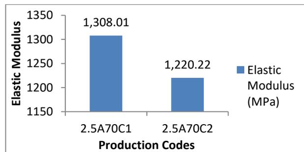
Figure 14. Comparison of elastic modulus values for different cement percentages
