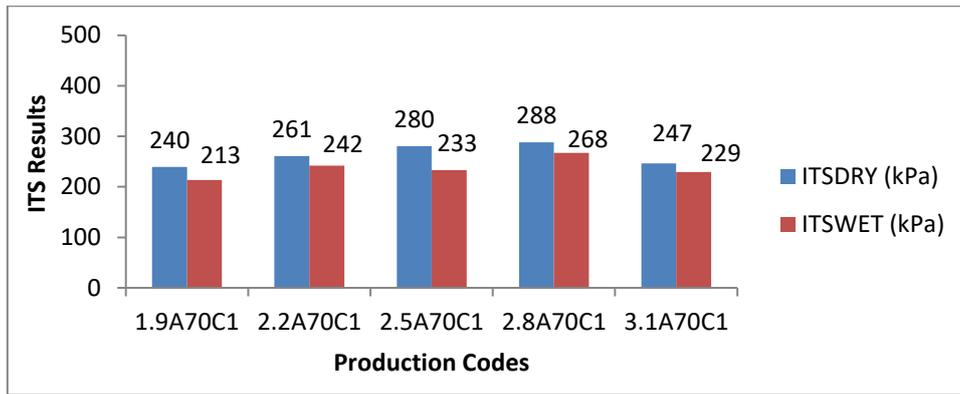
Figure 7. Comparison of ITSDRY and ITSWET values for different bitumen percentages
