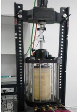
Figure 3. Resilient modulus test
