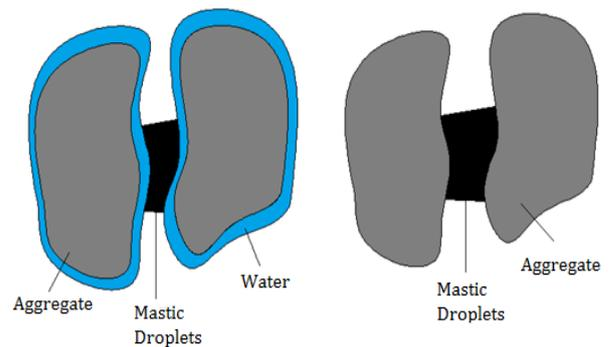
Figure 1. Foam bituminous cold mixture curing process
