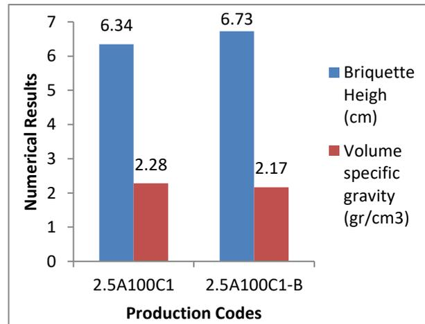
Figure 9. Comparison of briquette height and volume specific gravity values for different RAP materials
