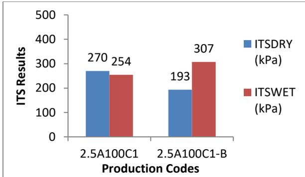
Figure 10. Comparison of ITSDRY and ITSWET values for different RAP materials
