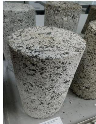
Figure 4. Unconfined compressive strength samples
