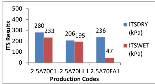
Figure 12. Comparison of ITSDRY and ITSWET values for different active fillers materials
