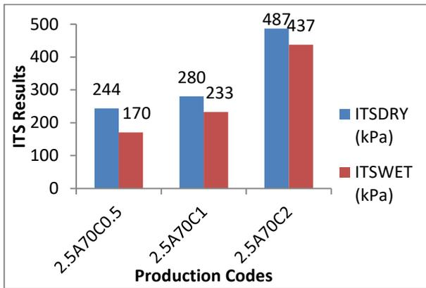
Figure 11. Comparison of ITSDRY and ITSWET values for different cement percentages
