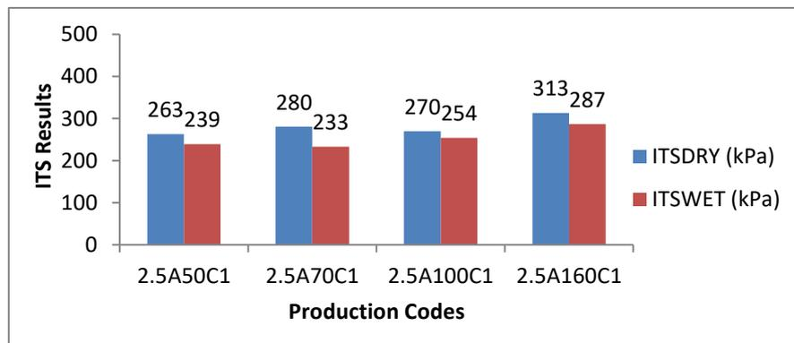
Figure 8. Comparison of ITSDRY and ITSWET values for different bitumen grades
