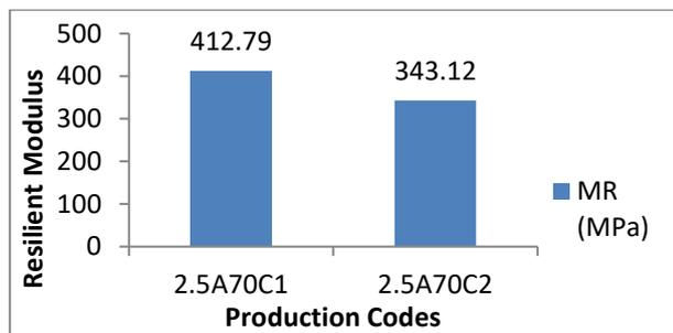
Figure 15. Comparison of resilient modulus values for different cement percentages
