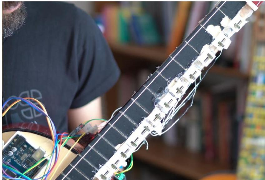
**Figure 16.** One-string prototype of the automatic microtonal guitar (Tolgahan Çoğulu, Personal Archive)
