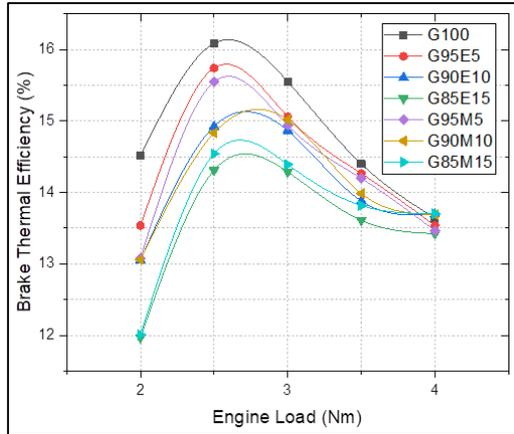
Fig. 6. Brake thermal efficiency (BTE) variation for all test fuels at different engine loads
