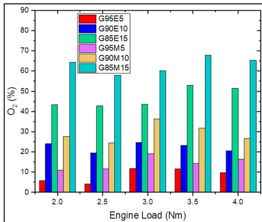
Fig. 11. O<sub>2</sub> variations of all blended fuels compared to gasoline for different load conditions
