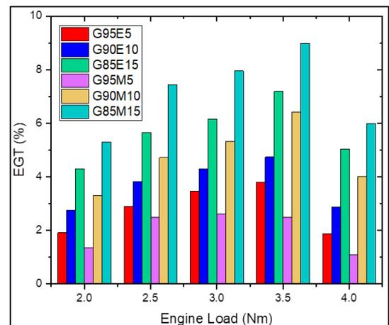
Fig. 9. EGT variations of all blended fuels compared to gasoline for different load conditions
