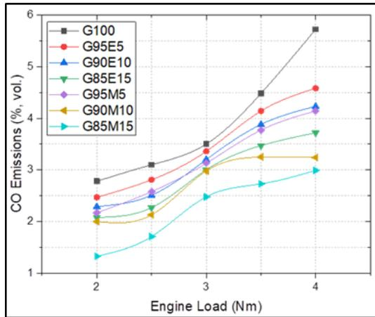
Fig. 14. CO variation for all test fuels at different engine loads
