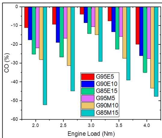
Fig. 15. CO variations of all blended fuels compared to gasoline for different load conditions
