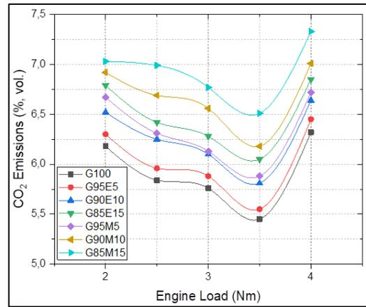
Fig. 12. CO<sub>2</sub> variation for all test fuels at different engine loads
