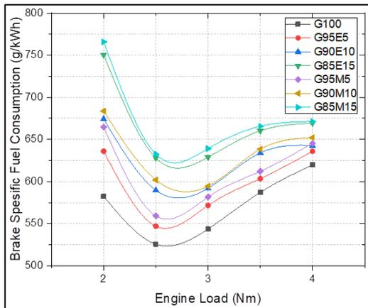
Fig. 2. Break specific fuel consumption (BSFC) variation for all test fuels at different engine loads
