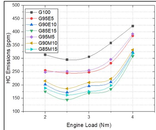
Fig. 16. HC variation for all test fuels at different engine loads
