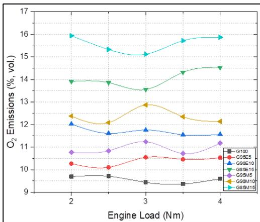
Fig. 10. O<sub>2</sub> variation for all test fuels at different engine loads
