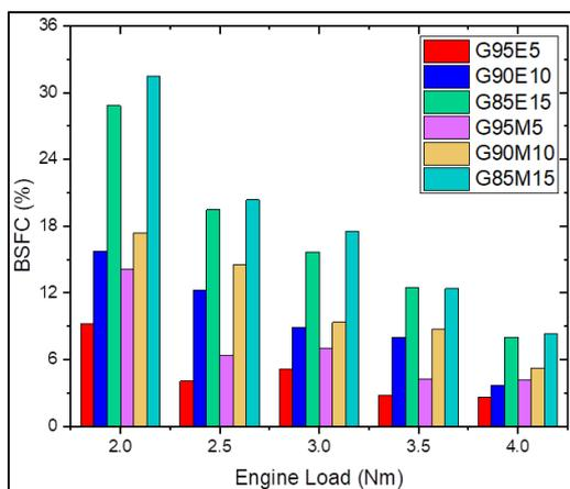
Fig. 3. BSFC variations of all blended fuels compared to gasoline for different load conditions
