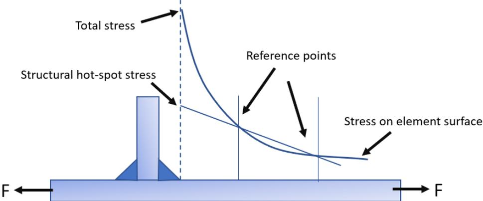
Figure 2. Definition of structural hot-spot stress (Hobbacher, 2016).
