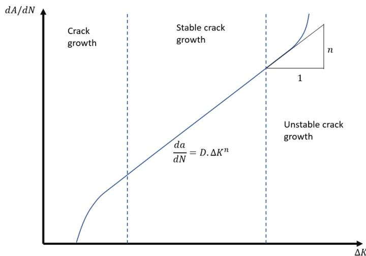
**Figure 6.** Crack growth curve (Fuštar et al., 2018).
