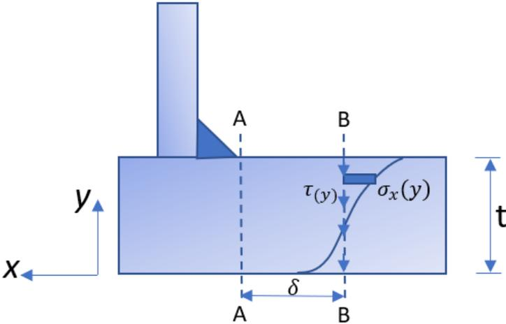
Figure 4. Structural stress calculation example (Dong, 2001).
