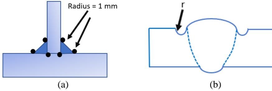
**Figure 5.** (a) Rounding of weld toe and root and (b) Rounding of a butt weld (Hobbacher, 2016).
