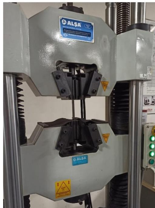
Figure 3. Tensile testing machine
