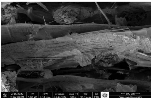
Figure 14. JBE composites at 70°C post cure temperature SEM micrograph
