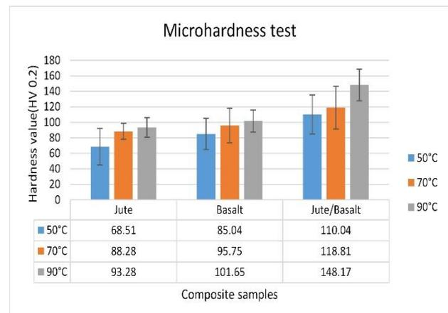
Figure 5. Hardness test results
