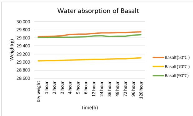
Figure 7. Water absorption analysis results of Basalt composite
