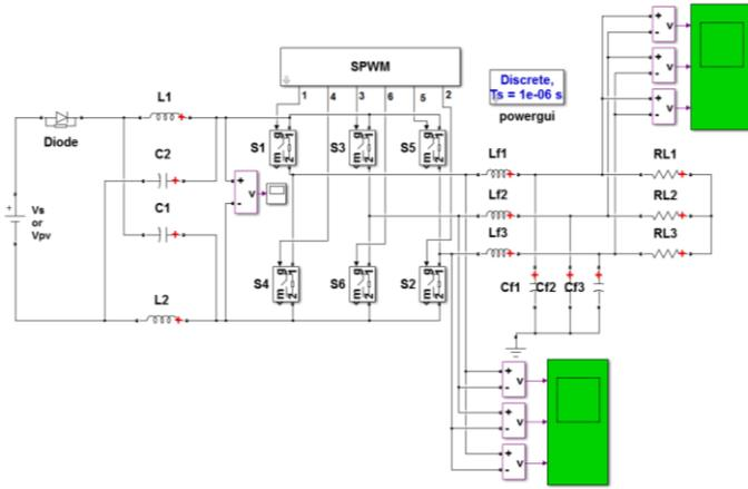
Figure 5. Matlab/Simulink model of the three-phase ZSI
