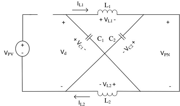
Figure 4. Equivalent circuit of the ZSI when the inverter is in the shoot through state
