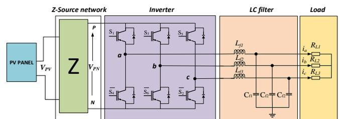
Figure 1. The topology of the three-phase ZSI
