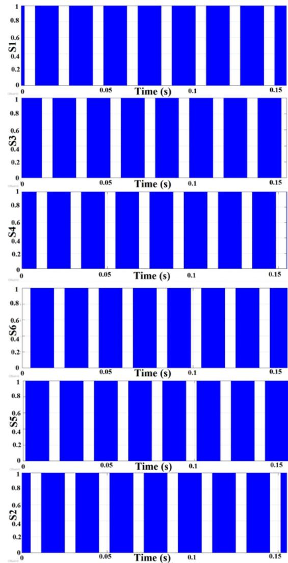
Figure 7. Simulink results of the three-phase simple boost control method of the switching signals
