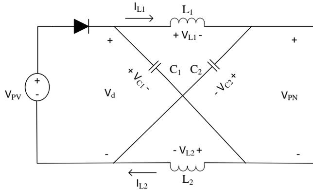
Figure 2. Equivalent circuit of the ZSI
