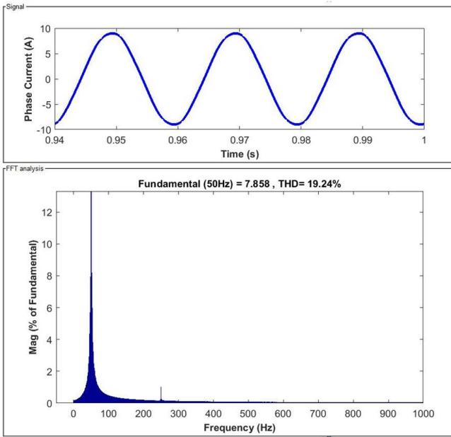
Figure 16. Phase current and harmonic spectrum of filtered output ( $M=0.9$  and  $T_0/T=0.1$ )
