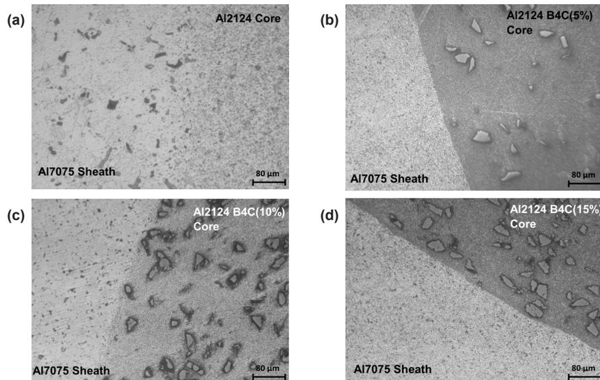
**Figure 3.** Optical microscope images of sheath-core boundary in hybrid composite materials, a) Al7075-Al2124 sheath-core boundary, b) Al7075-Al2124/ $B_4C$  (5%) sheath-core boundary, c) Al7075-Al2124/ $B_4C$  (10%) sheath-core boundary, d) Al7075-Al2124/ $B_4C$  (15%) sheath-core boundary.
