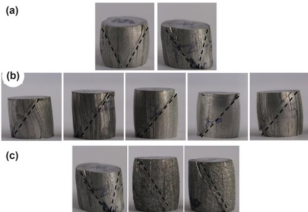
**Figure 9.** Fracture behavior of materials subjected to compression test, a) Semi-brittle fracture behavior of Al2124 and Al2124-B<sub>4</sub>C (5%), b) Brittle fracture behavior of Al7075, Al7075-Al2124, Al7075-Al2124-B<sub>4</sub>C (5%), Al7075-Al2124-B<sub>4</sub>C (10%) and Al7075-Al2124 (15%), c) Fracture behavior of Al2124-B<sub>4</sub>C (5%), Al2124-B<sub>4</sub>C (10%) and Al2124-B<sub>4</sub>C (15%).
