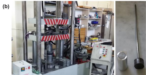
**Figure 2.** a) The extrusion billet produced with powder in tube method, b) Extrusion press and product (circular hybrid bar).
