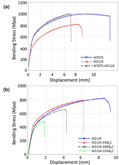
**Figure 4.** a) Bending stress-displacement ( $\sigma$ - $\delta$ ) curves of Al7075 and Al2124 rods and Al7075/Al2124 circular composite, b) Changing of  $\sigma$ - $\delta$  curves with  $B_4C$  ratio in circular composites.
