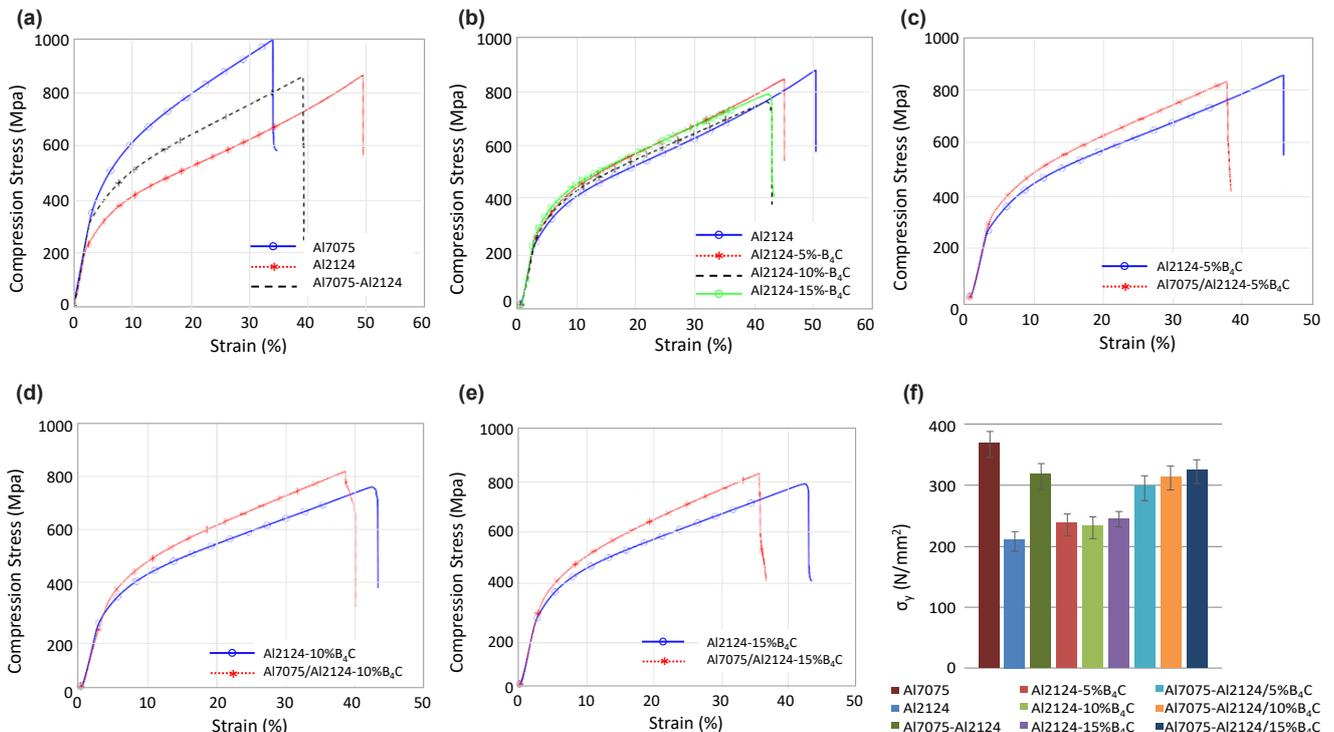
**Figure 7.** The changing of compression stress-strain % ( $\sigma$ - $\epsilon$ %) curves in a) Al7075, Al2124, and Al7075/Al2124 MM composites b) MM composite materials with B<sub>4</sub>C ratio, c) Hybrid and MM composites containing 5% B<sub>4</sub>C, d) Hybrid and MM composites containing 10% B<sub>4</sub>C, e) Hybrid and MM composites containing 15% B<sub>4</sub>C, f) changing of yield strength of sheathed and unsheathed composites.
