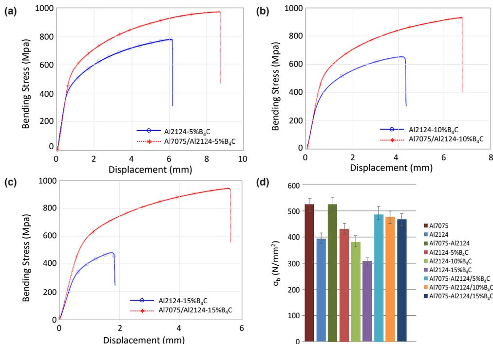
**Figure 5.** Changing of bending stress-displacement ( $\sigma$ - $\delta$ ) curves in a) unsheathed and sheathed composites containing 5%  $B_4C$ , b) unsheathed and sheathed composites containing 10%  $B_4C$ , c) unsheathed and sheathed composites containing 15%  $B_4C$ , d) changing of bending strength of sheathed and unsheathed composites.
