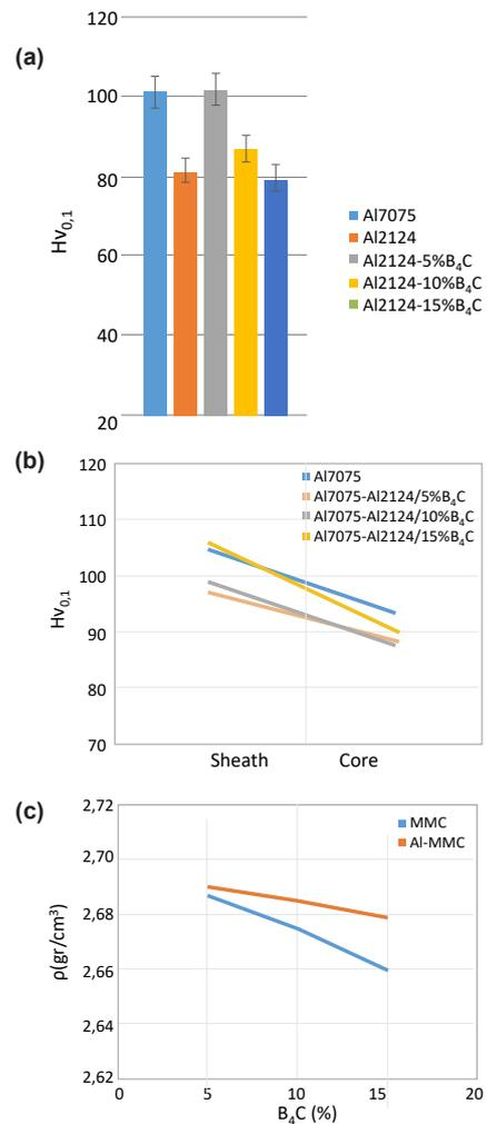
**Figure 10.** a) Changing of hardness values of Al7075, Al2124 and Al2124-B<sub>4</sub>C materials, b) Sheath-core hardness changing of sheath-core materials in hybrid composites, c) Density changing in Al2124-B<sub>4</sub>C and Al7075-Al2124/B<sub>4</sub>C composites depending on the B<sub>4</sub>C ratio.
