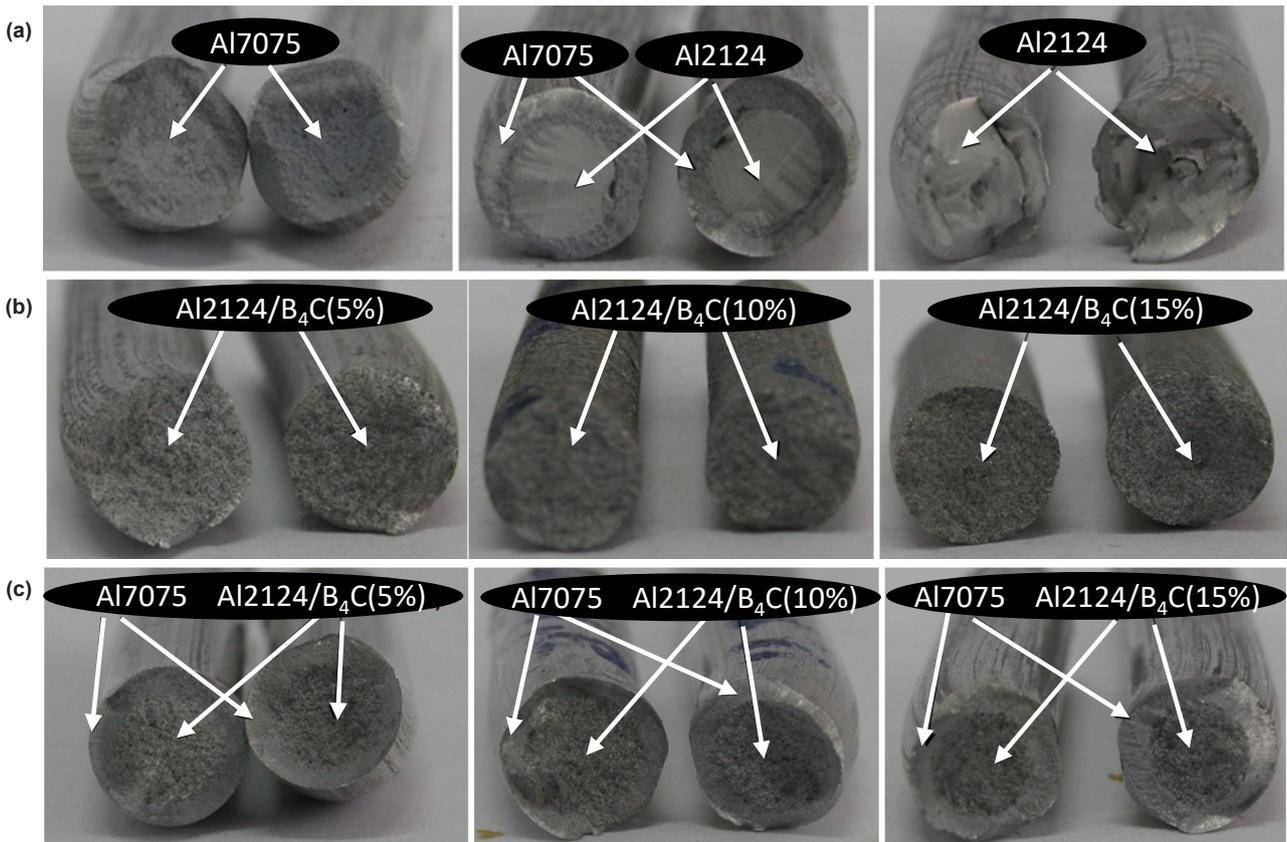
**Figure 6.** The fracture types of materials subjected to bending test, a) Al7075, Al7075-Al2124 and Al2124, b) Al2124-B<sub>4</sub>C (5%), Al2124-B<sub>4</sub>C (10%) and Al2124-B<sub>4</sub>C (15%). c) Al7075-Al2124-B<sub>4</sub>C (5%), Al7075-Al2124-B<sub>4</sub>C (10%) and Al7075-Al2124-B<sub>4</sub>C (15%).
