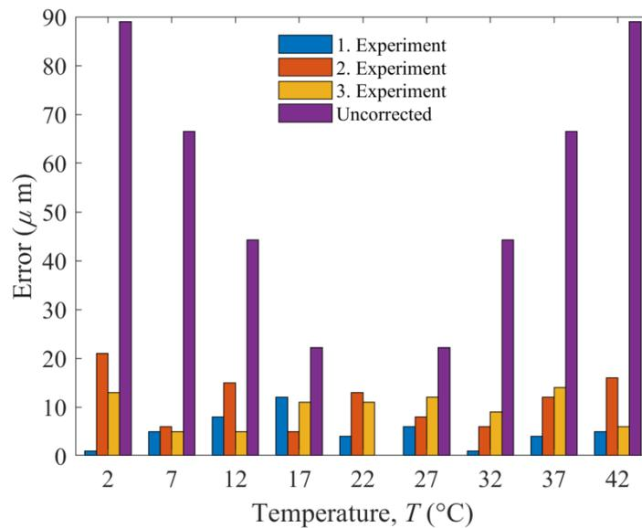
**Figure 13.** Al7075(T6) temperature-dependent error measurement for x=60mm
