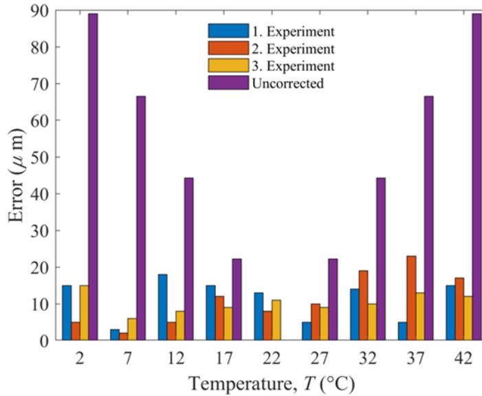
**Figure 14.** Al7075(T6) temperature-dependent error measurement for x=100mm
