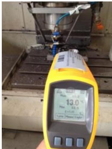
**Figure 9.** Infrared temperature gauge
