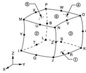
**Figure 3.** Element type SOLID186 used in FEM analyzes.
