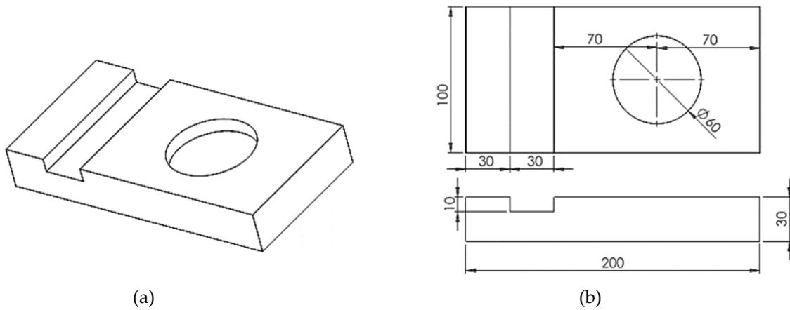
**Figure 4.** Model Part dimensions (a) full model (b)side and top view
