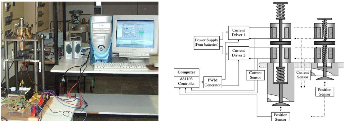
b. Schematic diagram and picture of dynamic test setup
