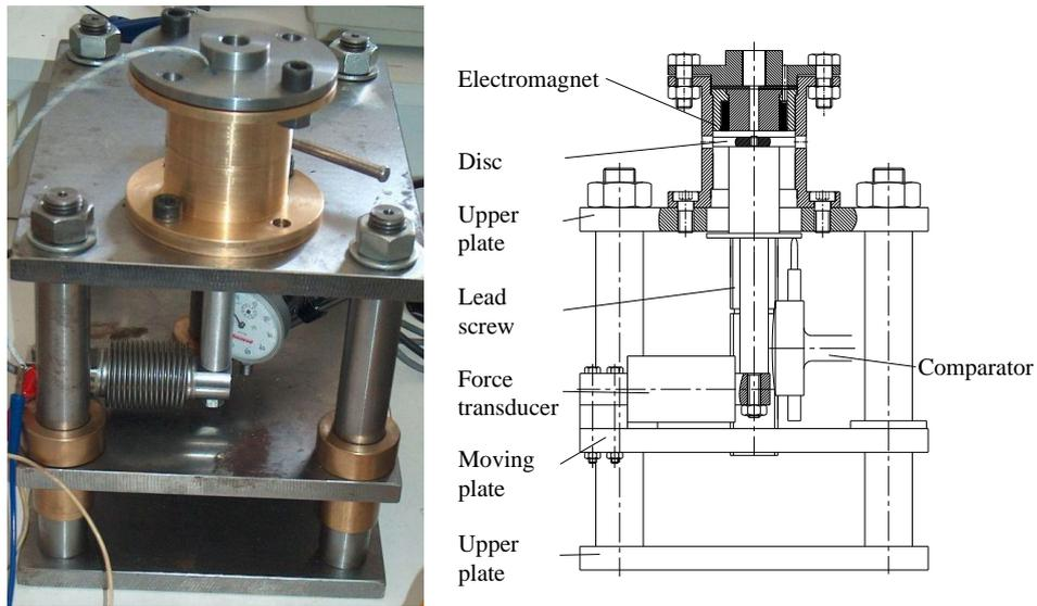
a. Static test setup
