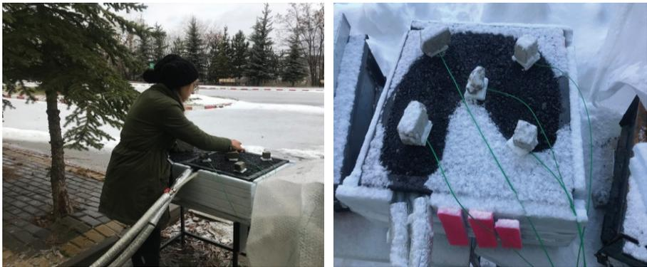
Figure 3 - Measurements of asphalt surface temperatures with thermocouples
