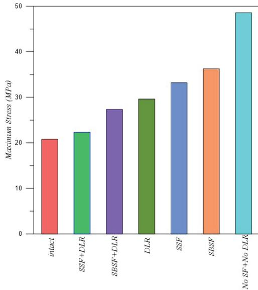
**Figure 9:** Maximum stress in the talus for models.
