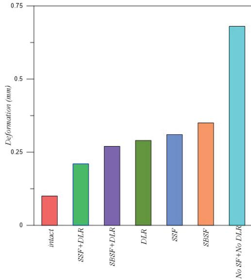
**Figure 8:** Deformation in the talus for models.
