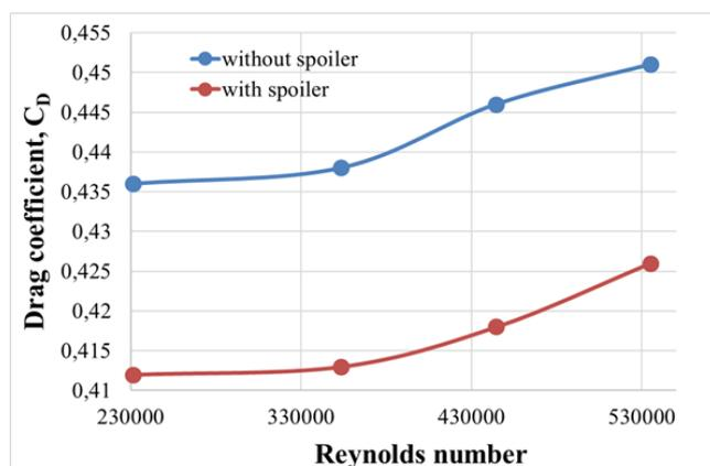
Fig. 4. Drag coefficient curve at different vehicle speed for spoiler application
