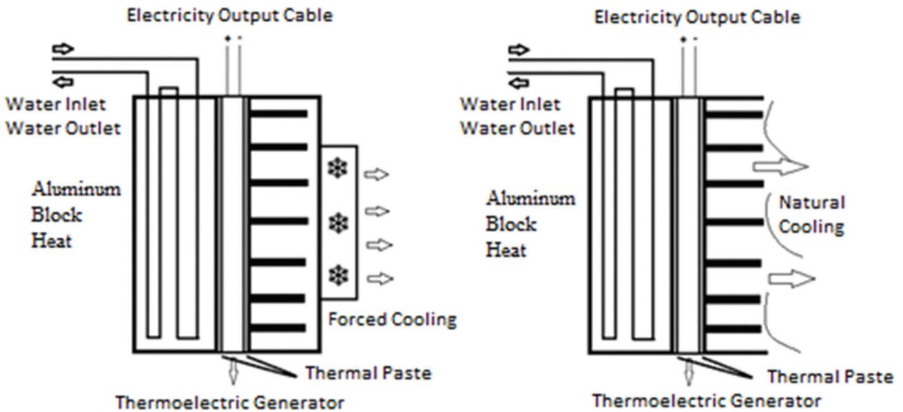
Figure 4. Forced and atmospheric cooled thermoelectric generator.
