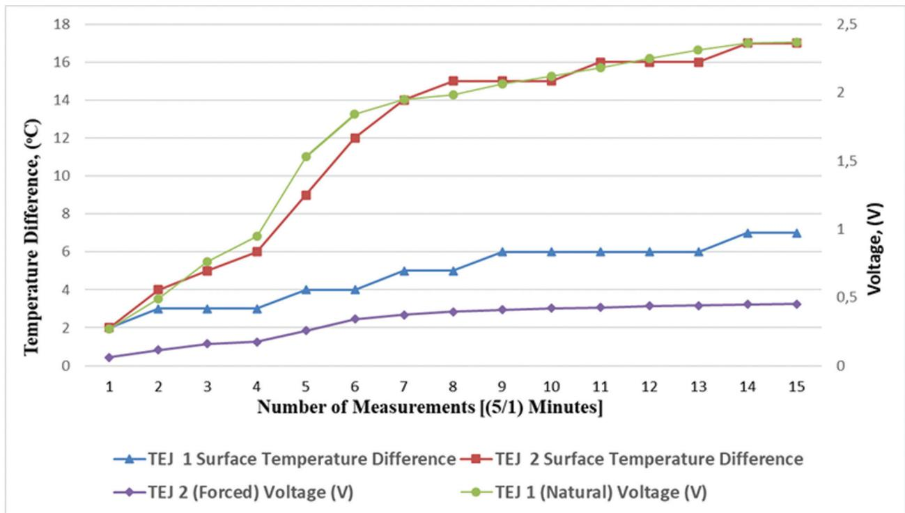
Figure 11. Electricity generation due to temperature difference between TEG’s surfaces.
