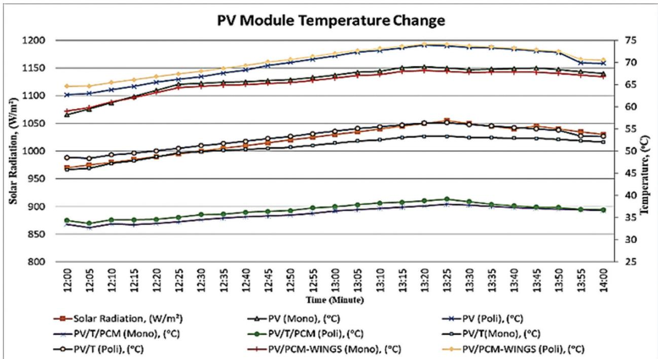
Figure 7. Change in module temperature due to solar radiation (26.08.2019).
