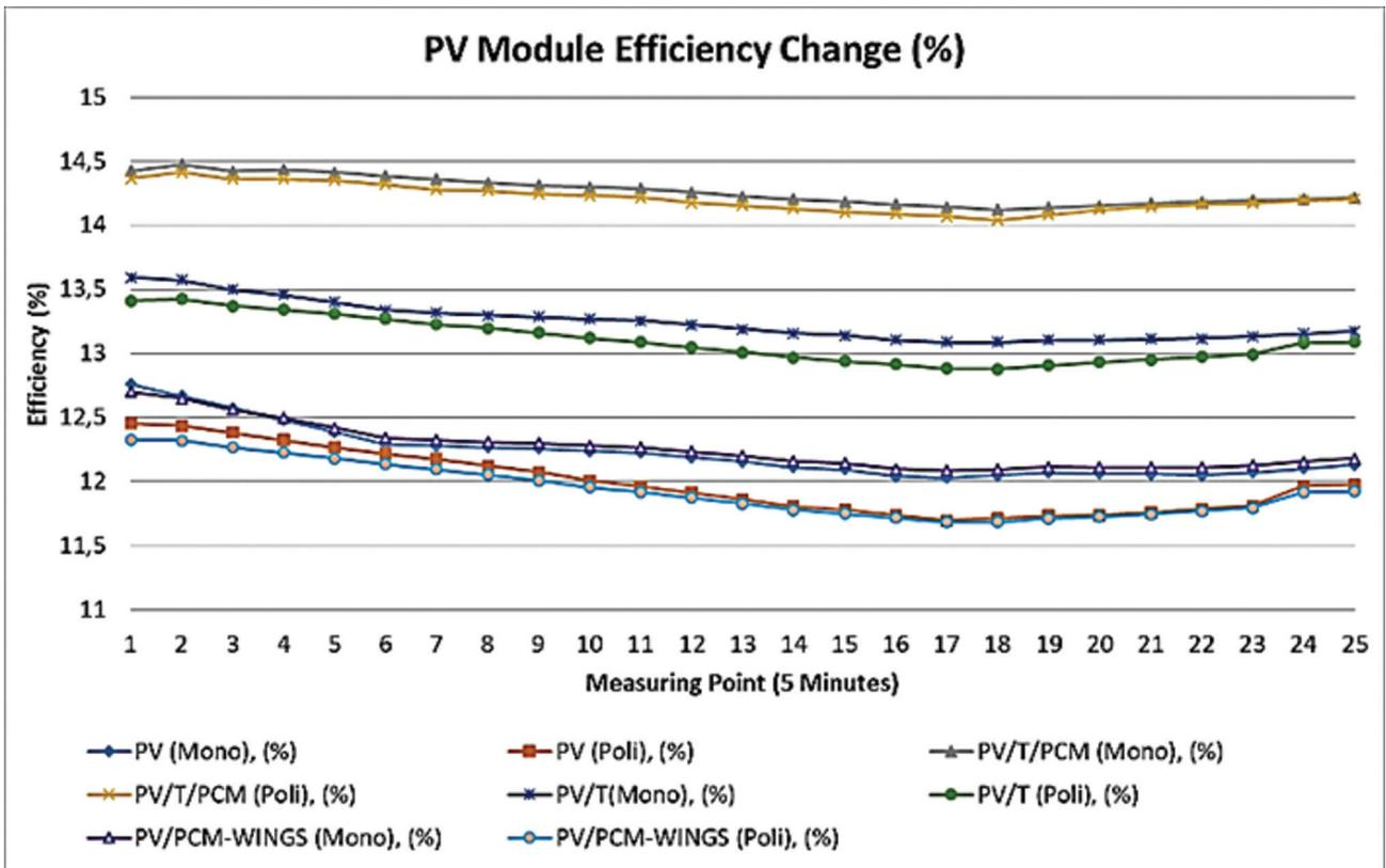
Figure 10. Efficiency changes of PV modules.
