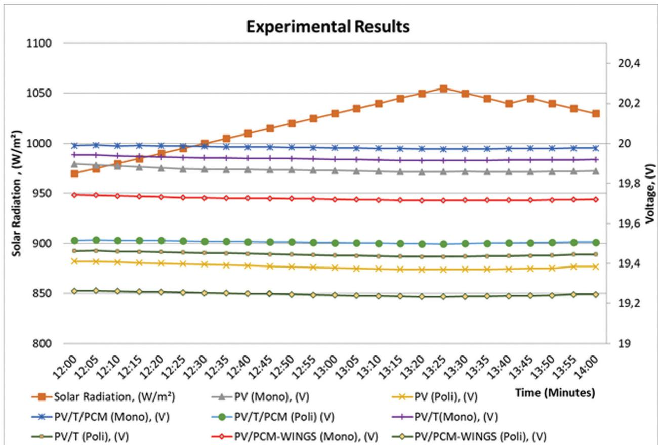
Figure 8. Voltage values due to solar radiation.
