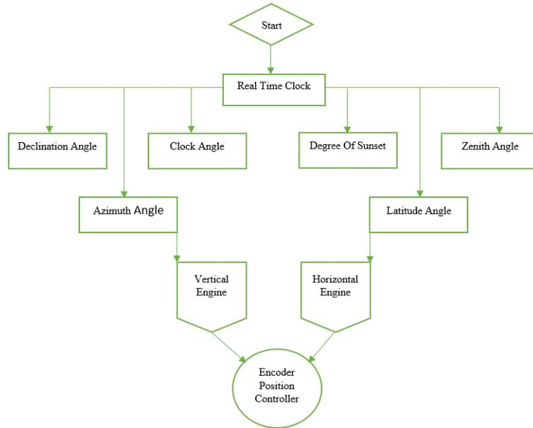
Figure 8. Flow diagram using Delta PLC "WPL soft".
