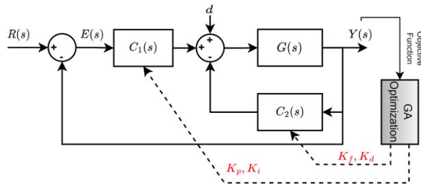
Figure 2. Block diagram of proposed optimization scheme.
