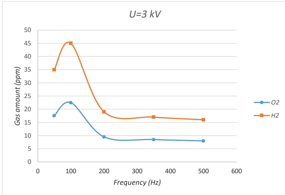
**Figure 3.** Frequency-Gas Quantity characteristic taken at constant voltage  $U=3$  kV
