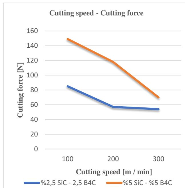
**Figure 3:** The variation of cutting force with cutting speed (f: 0.1mm/rev).
