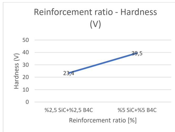
**Figure 11.** The variation of hardness with reinforcement ratio (Load:1000 gf)
