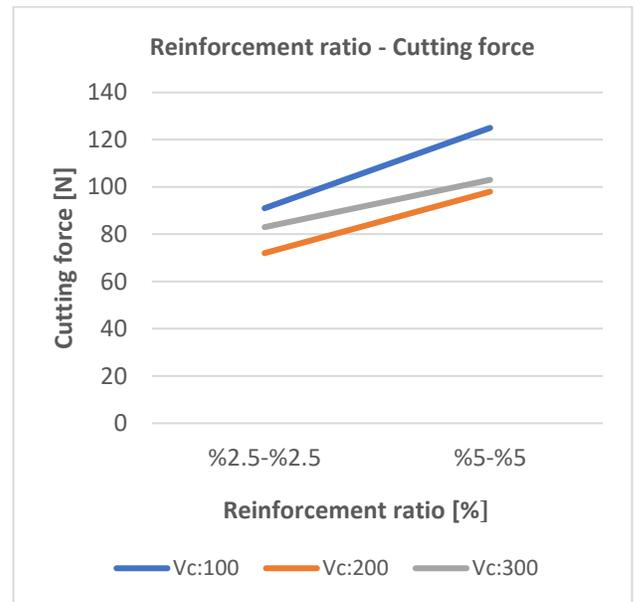
Figure 6: The variation of cutting force with reinforcement ratio ( $f$ : 0.1mm/rev)
