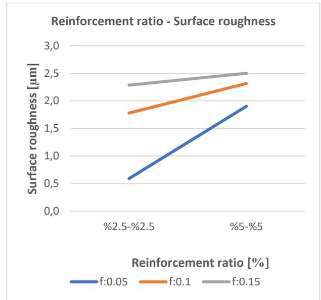
**Figure 10:** The variation of surface roughness with reinforcement ratio (Vc:100 m/min)
