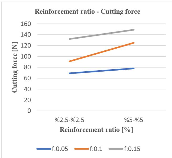
Figure 5: The variation of cutting force with reinforcement ratio ( $V_c$ : 300m/min)
