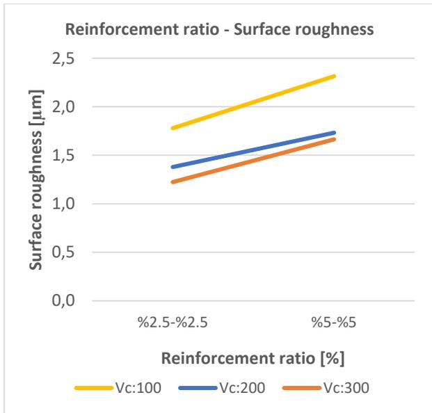
**Figure 9:** The variation of surface roughness with reinforcement ratio (f:0.1 mm/rev)
