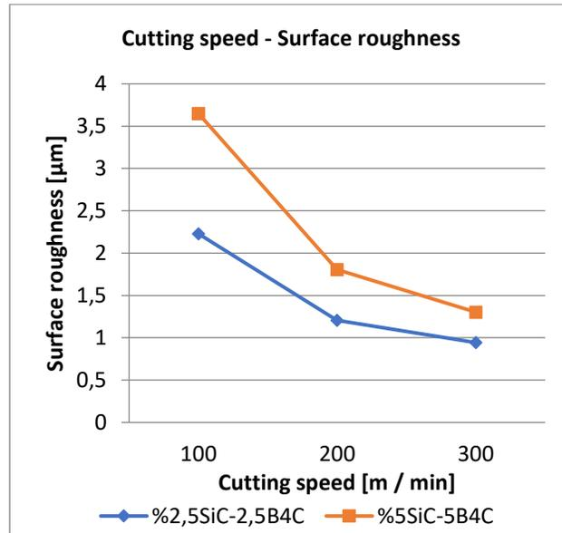
**Figure 7:** The variation of surface roughness with cutting speed ( $f:0.1 \text{ mm/rev}$ )
