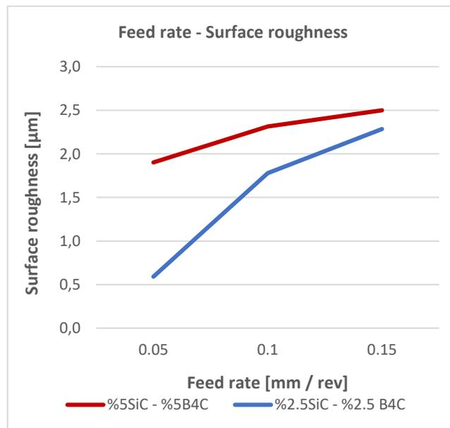
**Figure 8:** The variation of surface roughness with feed rate ( $V_c:100\text{m/min}$ )
