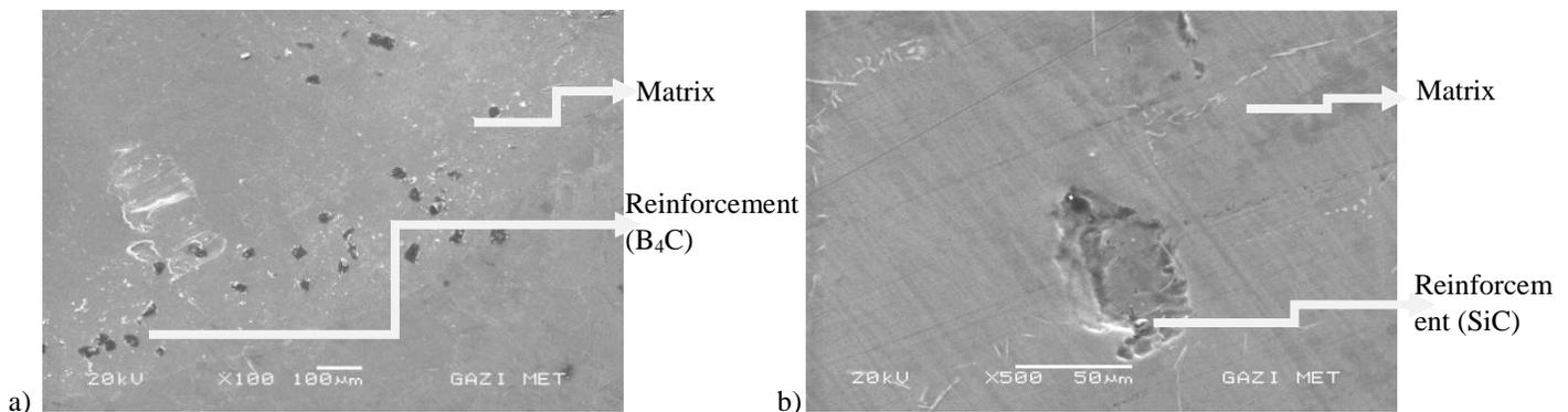
**Figure1:** Images of MMC materials reinforced with 5% SiC- 5% B<sub>4</sub>C in SEM
