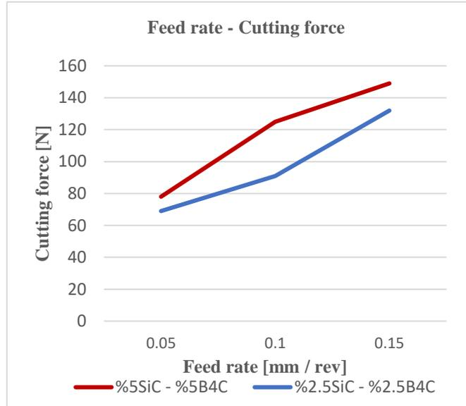
Figure 4: The variation of cutting force with feed rate ( $V_c$ : 300m/min)
