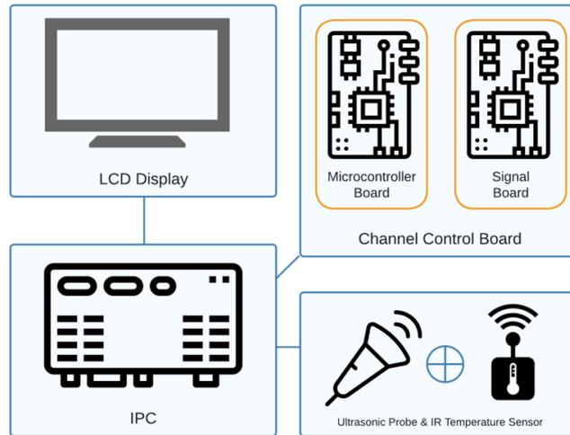
**Figure 1.** A Complete block diagram of the fuzzy logic based ultrasonic therapy device H/W
