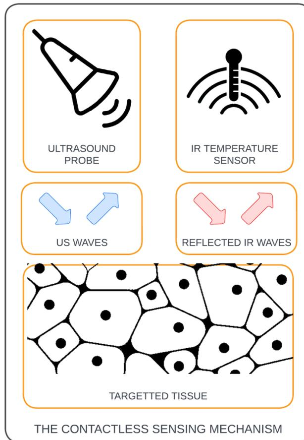
**Figure 3.** The contactless sensing for ultrasonic energy absorbed on tissue with IR temperature sensor.
