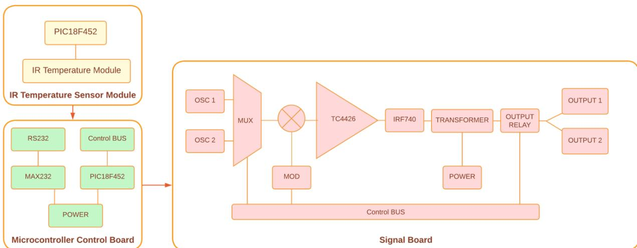
**Figure 2.** The Detailed Block Diagram of H/W Structure of the Ultrasonic Therapy Device
