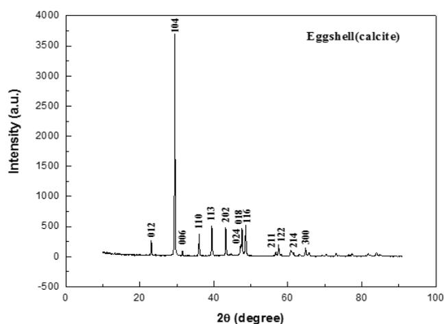
**Figure 1:** XRD analysis for egg shell (calcite).
