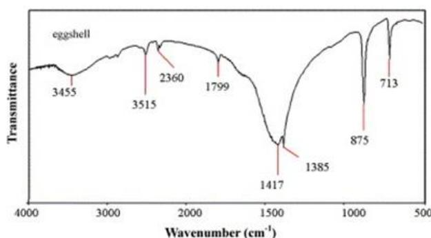
**Figure 3:** FT-IR spectra of egg shell (calcite).
